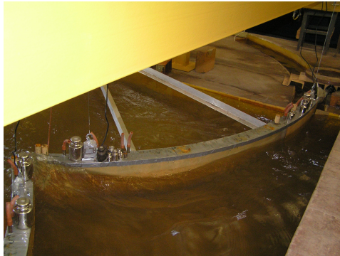
(a) A photo taken during the physical model test for the main case with 0^\circ wave incidence at the gate
