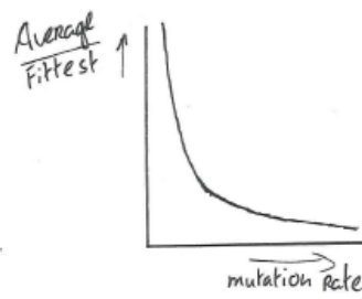
Figure C.3: The correlation between the ratio of the average and fittest score to the mutation rate.
