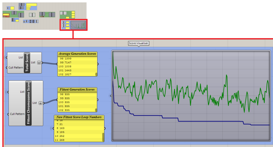
Figure 4.19: Optimisation process graph, showing the fitness scores during looping on a logarithmic scale.
