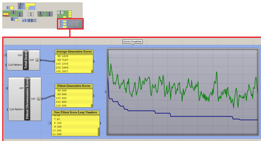
Figure C.2: Blue line represents the fittest score and the green line the average generation score.
