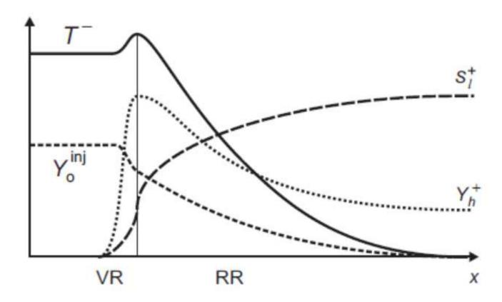
The thin region VR is dominated by vaporization and the much wider region RR is dominated by MTO reaction (with slow condensation). The VR is much thinner than the RR, because it is assumed that vaporization rate is much faster than the reaction rate
