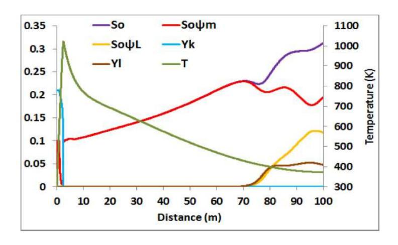
t=1.26x10<sup>8</sup> sec, initial medium component fraction of  $\psi_m^{\text{ini}}$ =0.8 , base pressure (10 bar) and higher injection rate 3xu<sup>inj</sup>
