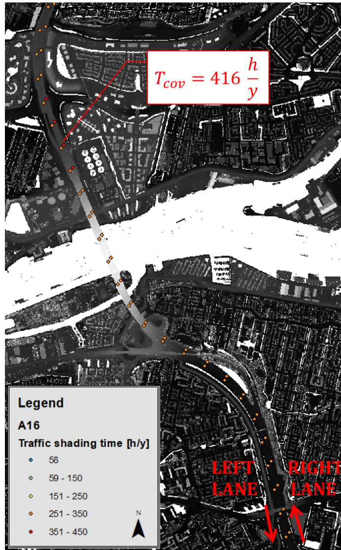
Figure 5.13: Brienenoordbrug in the East of Rotterdam (1:20.000). The points along the road indicates the traffic coverage factor in the specific location
