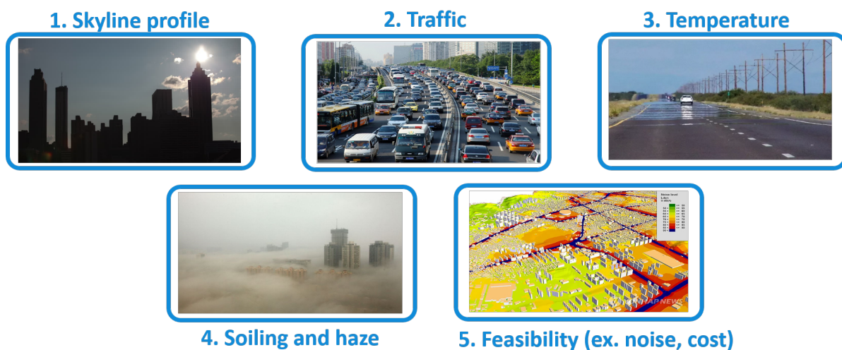
Figure 4.1: When modelling solar road systems, five main aspects should be considered: the shading caused by the elevated skyline, the shading caused by vehicles, the output reduction due to operational temperature, the performance drop due to soiling effect and variation of irradiance due to haze and pollution, and the feasibility of the installation. The latter includes considering noise generation, costs, etc.
