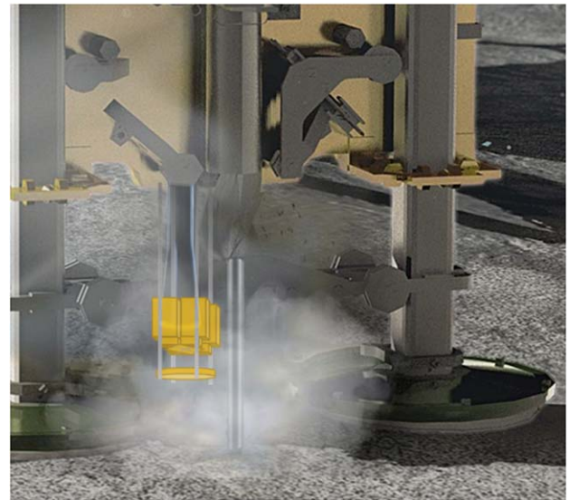
Figure 8. Artist rendition of a low-SWaP system deployed next to a drill affixed to the side of a Philae-like comet landing craft (Di Lizia et al. 2016). Immersion of the open cavity structure in the plume allows for instantaneous monitoring of lost volatiles during sampling.
