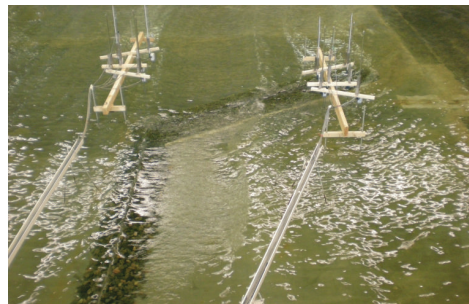
Figure 3.10: Reduced diffraction effects observed due to the additional rubble mound
