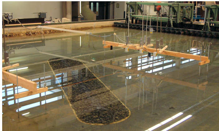
Figure 2.10: Wave gauges mounted on a longer frame
