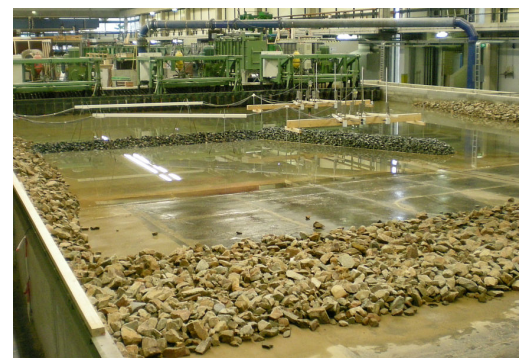
(b) View of the additional rubble mound in the dry wave basin
