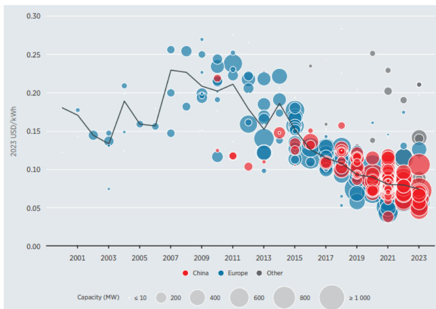
Figure 2.6: Project costs and in 2023 $ / kWh and global weighted averaged of newly installed capacity. Reproduced from [3]
