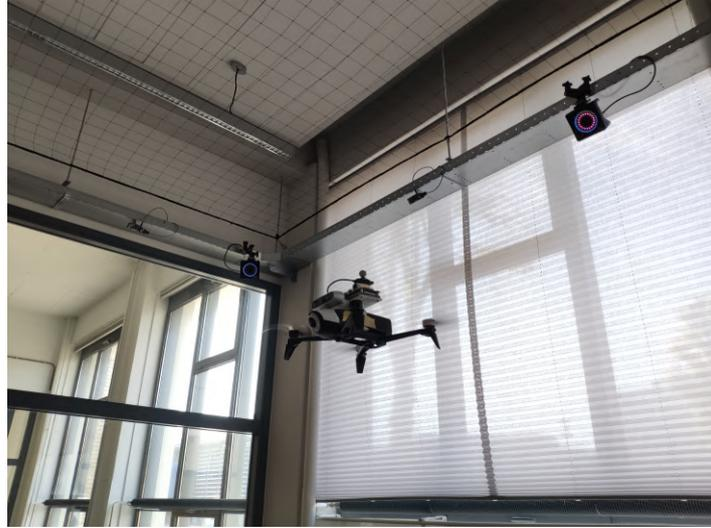
**Figure 4-3:** Parrot Bebop2 with a forward-looking visual-inertial sensor and an onboard computational unit. The reflective markers are equipped for collecting ground truth.
