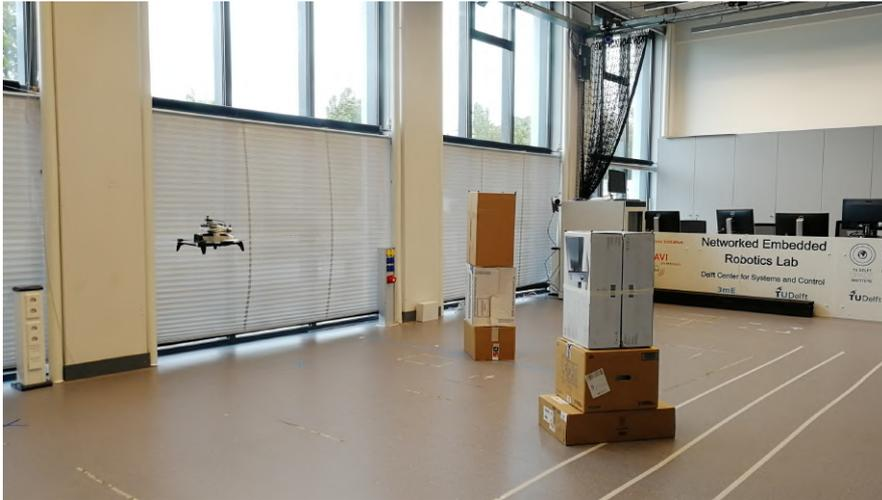
**Figure 5-6:** The snapshot of the experiment setup: MAV is hovering in front of two static obstacles.
