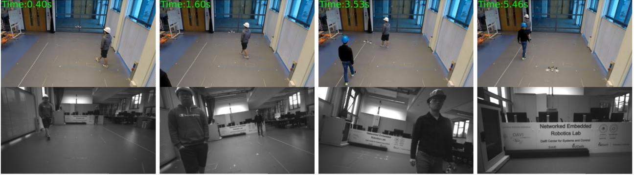
Fig. 5: A sequence of images during the experiment Scenario 1. The MAV is required to fly from a start point to an end goal while avoiding two walking humans. Top: Snapshots of the experiment. Bottom: On-board camera grayscale images.
