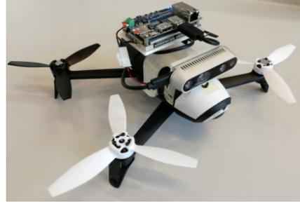
Fig. 4: MAV used in the experiments. It is equipped with an NVIDIA Jetson TX2 Module for all on-board computation, an Intel RealSense Depth Camera D435i dually for visual-inertial odometry and depth image sensing.
