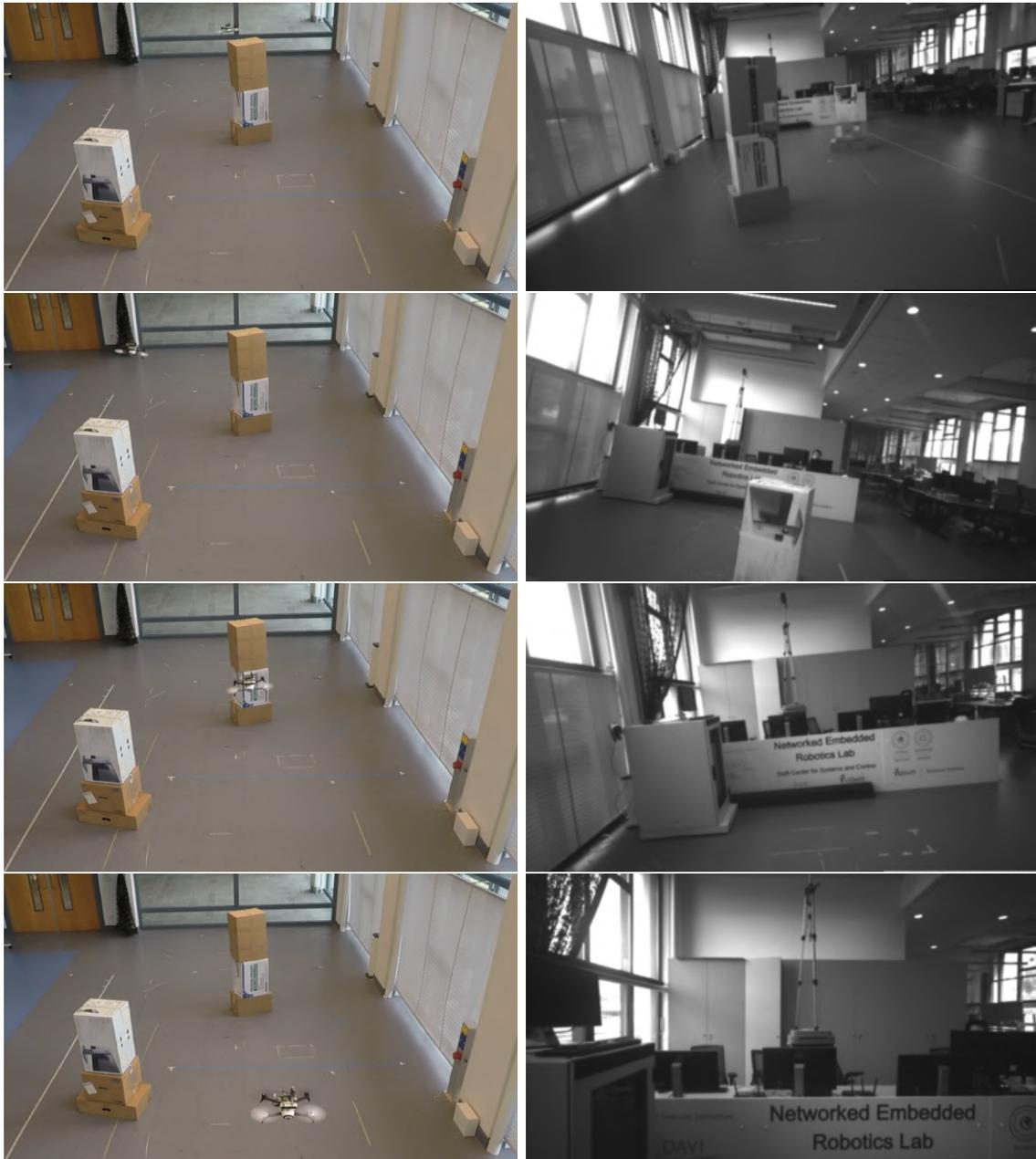
**Figure 7-1:** A sequence of images (from the top to the bottom) during the experiment in scenario 1 with static obstacles. The snapshot (left) is captured by the external camera, while the onboard grayscale image is taken by the MAV onboard camera.
