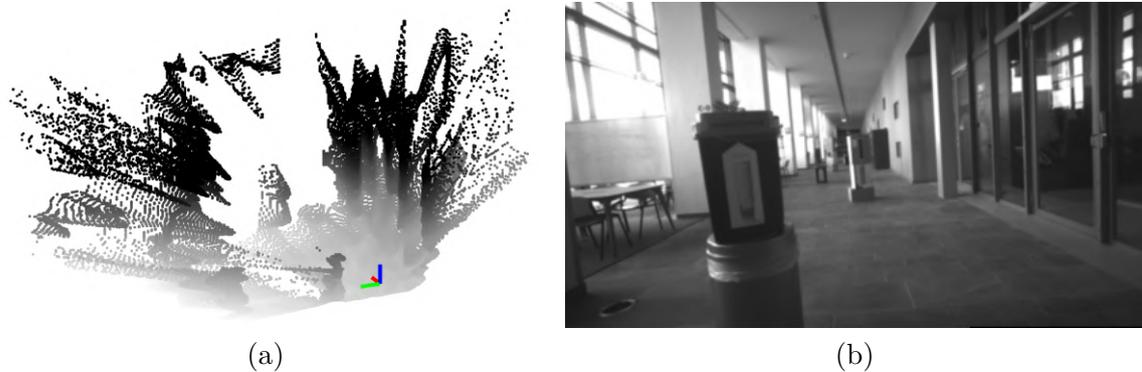
**Figure 5-1:** (a) A three-dimensional point cloud generated by RealSense Depth Camera D435i and (b) its corresponding grayscale image. Points are marked by colors according to their heights.
