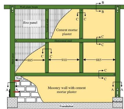
Figure 2.21: Details of a typical Assam type house (Chand et al., 2020a)
