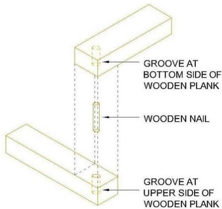
Figure 2.10: Connection of perpendicular wooden planks by wooden dowel (Rahul et al., 2013)
