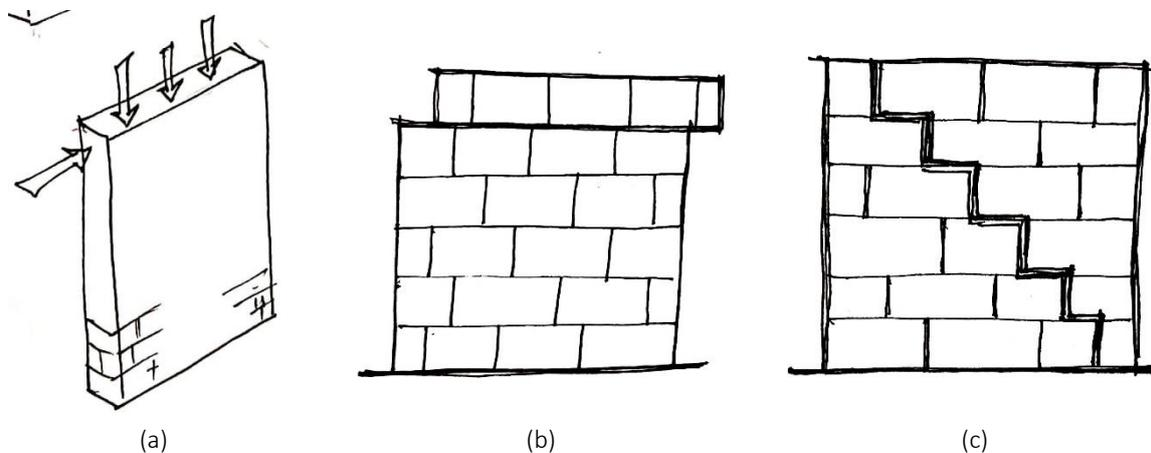
Figure 3.2: (a)-(c) In-plane failure mechanisms
