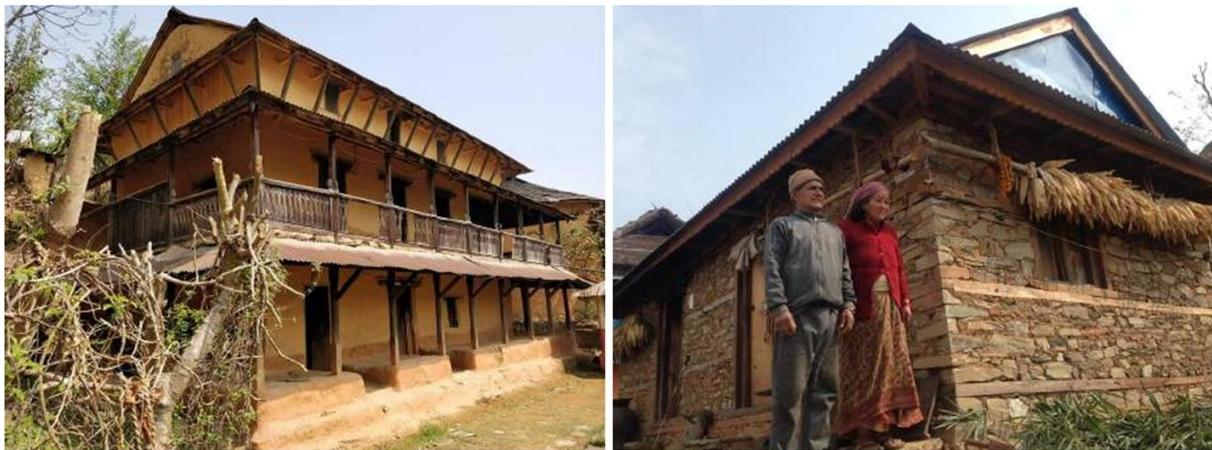
Figure 5.1: Stone masonry houses with seismic resistant features of timber elements
