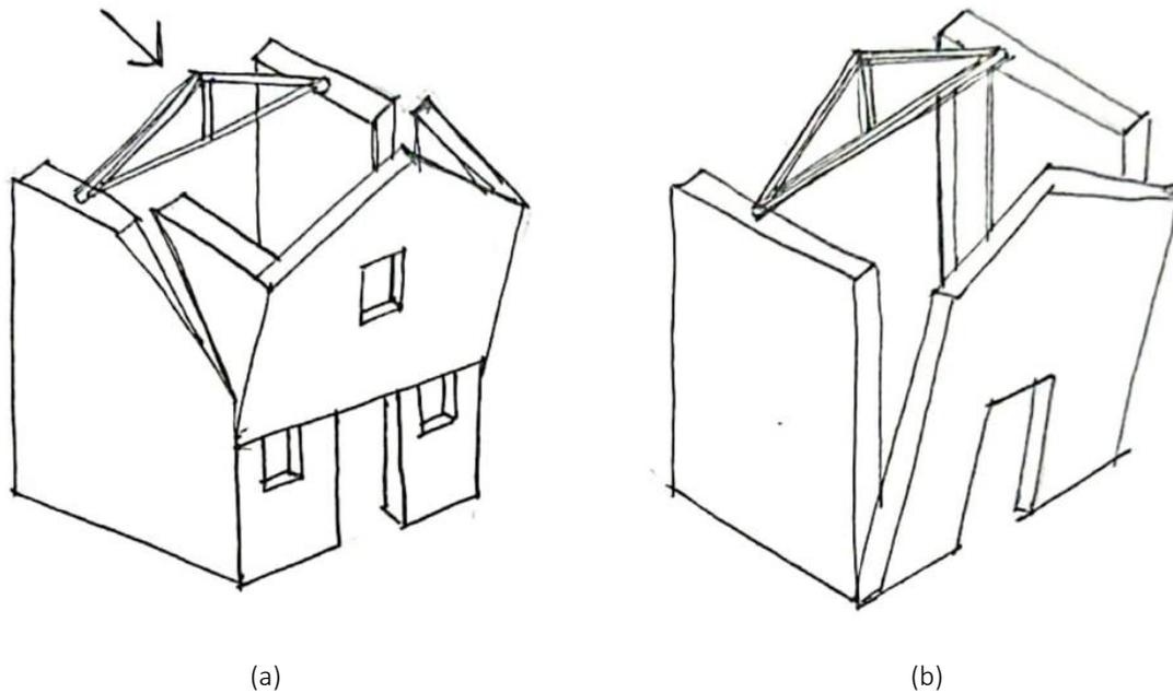
Figure 3.3: Out-of-plane failure mechanisms
