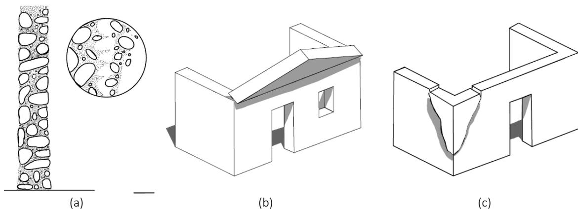
Figure 3.1: Local failure mechanisms
