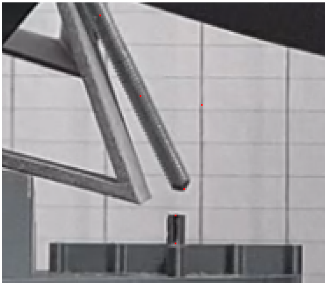
Figure F.2: A zoomed-in view of the upper (PMMA) screen showing two red marked pixels on the fixed reference point, three on the pendulum's central axis and one on a gravity indicator (two markings on the gravity indicator are located outside of this view).
