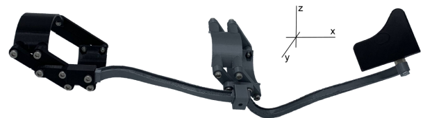
Fig. 7. The 3D printed prototype with forearm, wrist and hand support connected by the spatial beams. Retrieved from [21].
