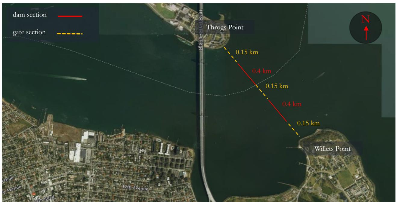
Figure 6.6 | Barrier layout between Throgs point – Willets Point.
