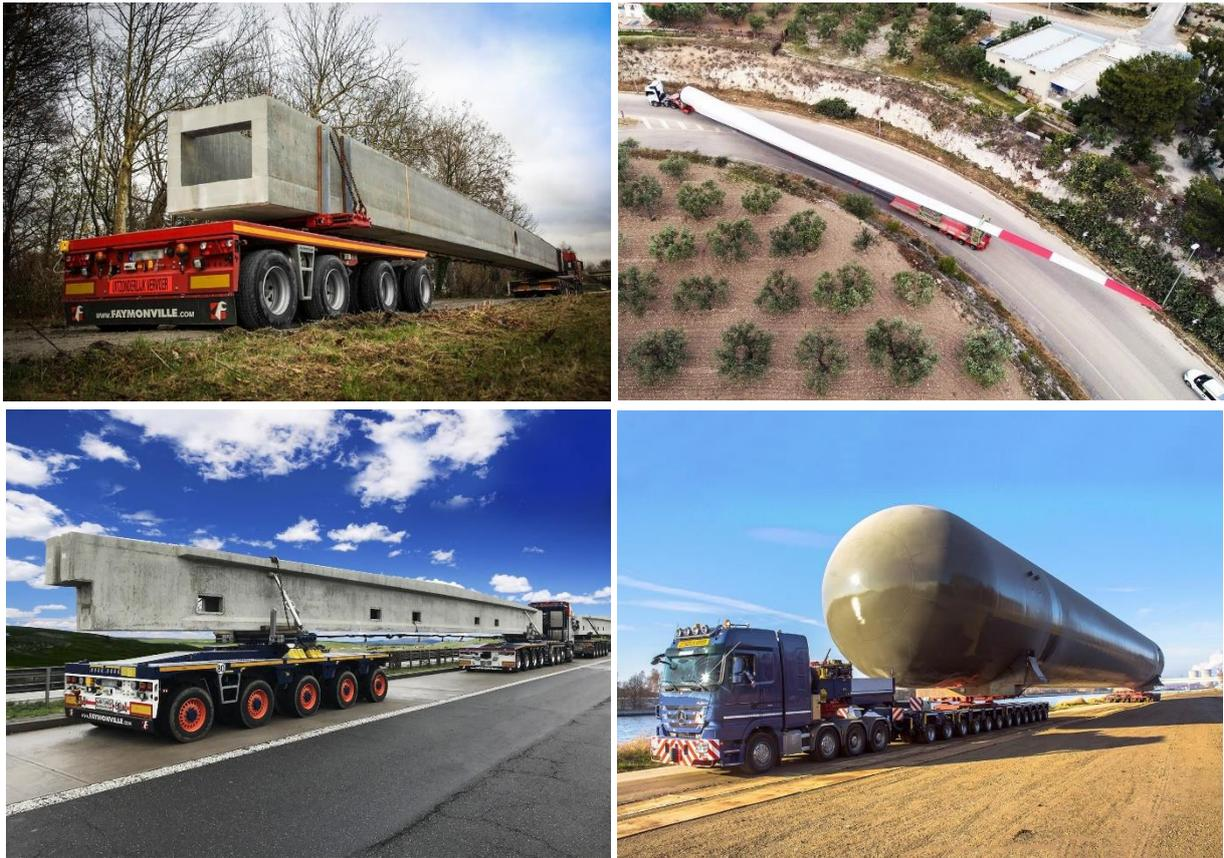
Figure 6.10 | Long and heavy transport equipment including a 70 m long wind turbine blade (Faymonville, n.d.).
