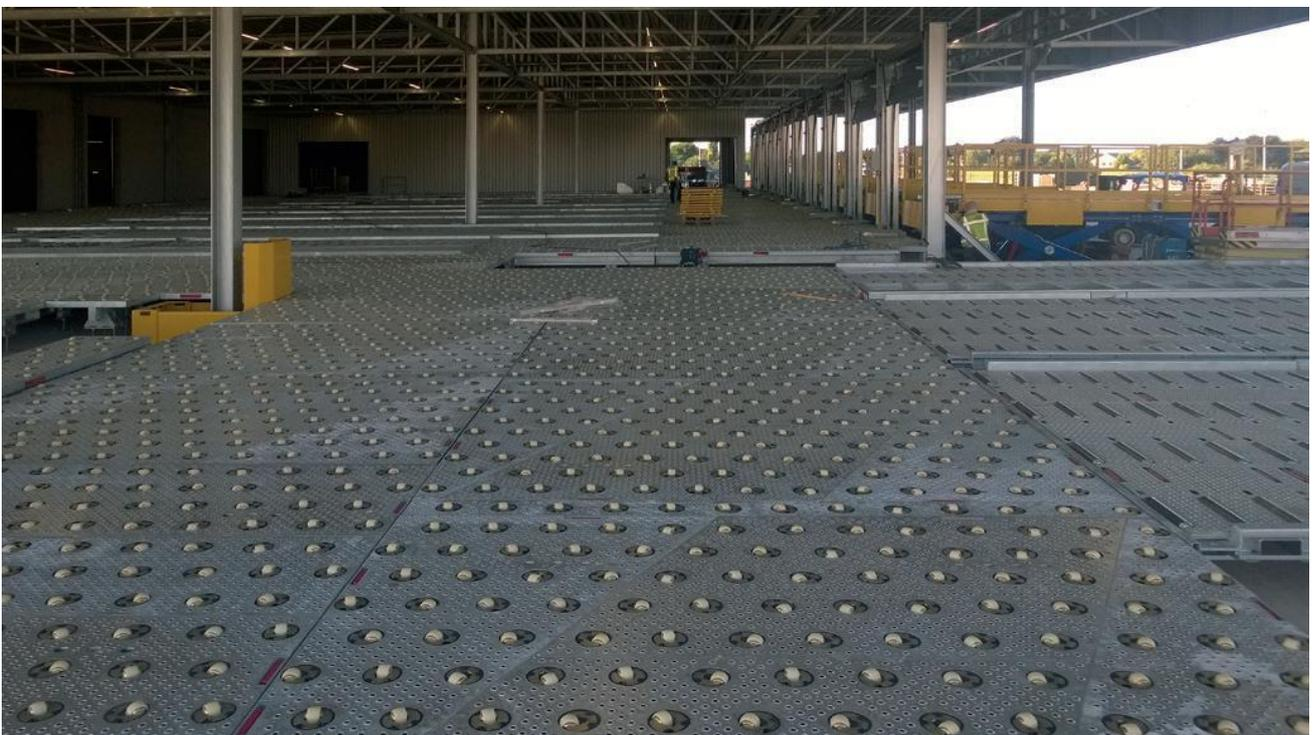
Figure 6.15 | Roller deck for transporting segment (AirportTechnology, 2016).
