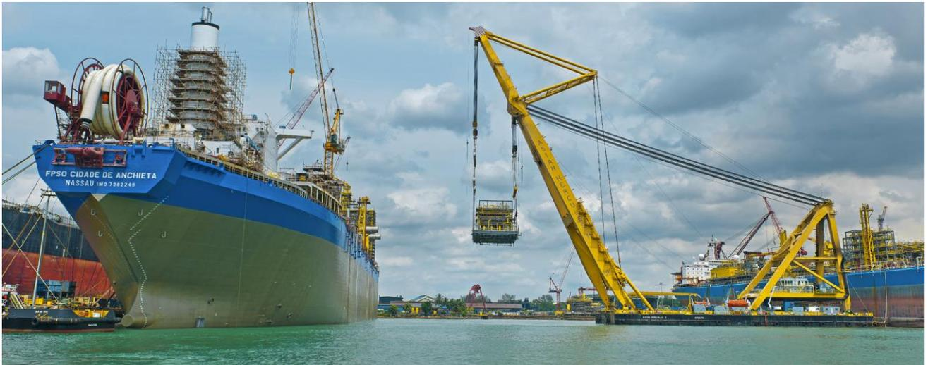
Figure 6.14 | Asian Hercules II vessel with a lift capacity up to 3200 tons (Royal Boskalis Westminster N.V., n.d.).
