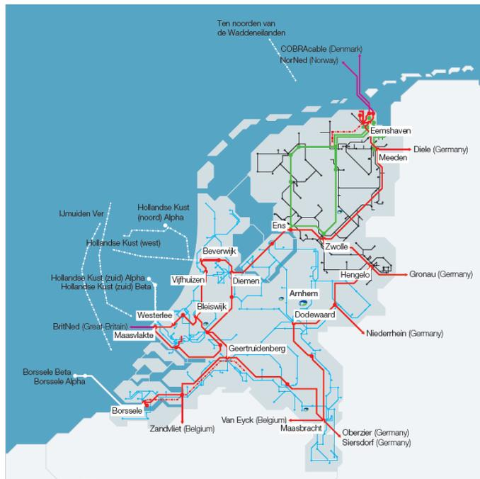
Figure 9.1: The Dutch transmission grid
