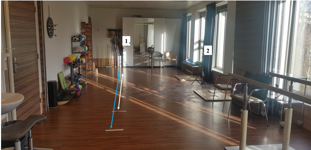
Figure 11: Set-up in the physical therapy room at Basalt The Hague. 1 and 2 show the placement of the phone cameras on tripods. The blue arrow is the 7 meter distance lines which the subjects have to walk. The white arrow shows the 5 meter distance which is recorded and analysed.
