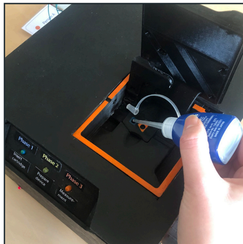
13). Insert the immersion oil on the blue square of the cartridge.
