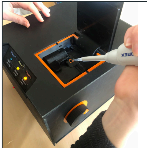
21). Pipet the sample on the orange triangle at the cartridge.
