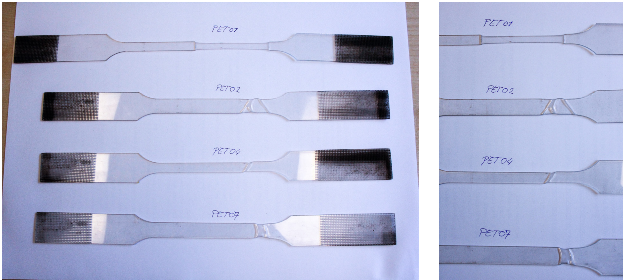
Figure C1.10: The pull test specimens after the pull test. The righter figure enlarges the critical area.
