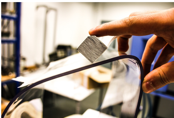
Figure P1.22: A knife-edge is used to apply the vertical displacement to the physical model during testing. This knife-edge is kept in its place with the aid of a double-sided tape.
