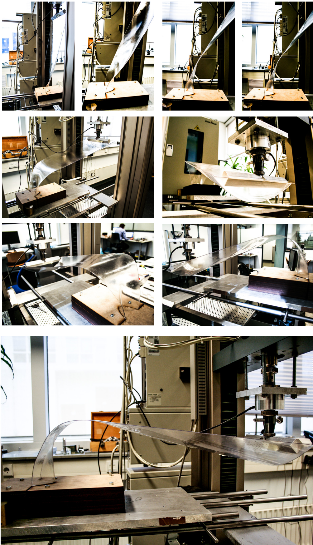
Figure C1.6: The physical model is being tested by a compression bench, which measures the vertical displacement and the required force simultaneously.
