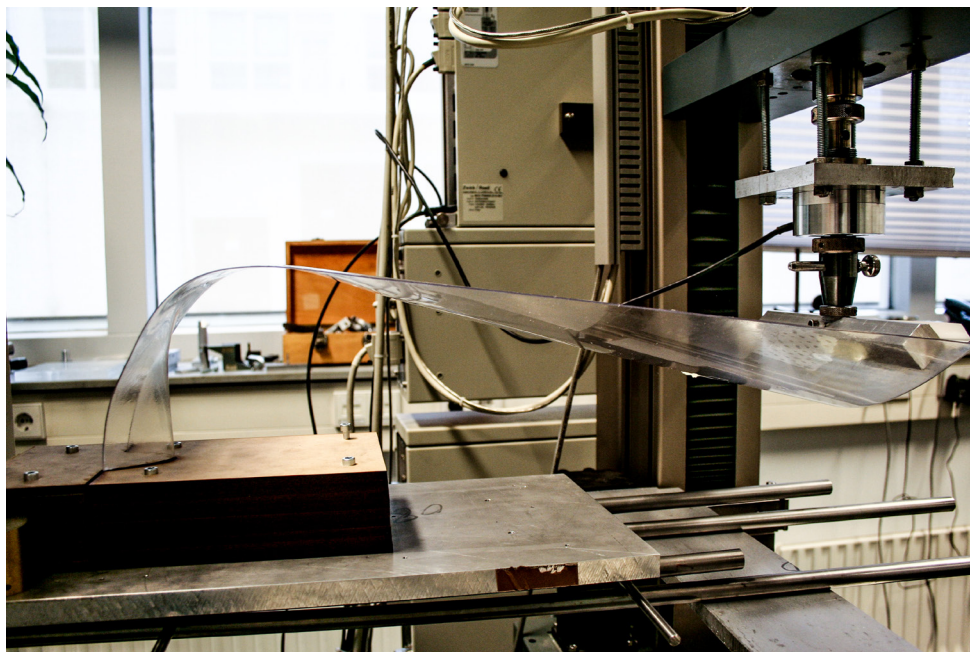
Figure P2.23: The physical model during a compression test. The compression bench displaces itself in a vertical sense and measures the vertical displacement and the force simultaneously. The foundation of the model is displaced in horizontal direction due to straight rollers.
