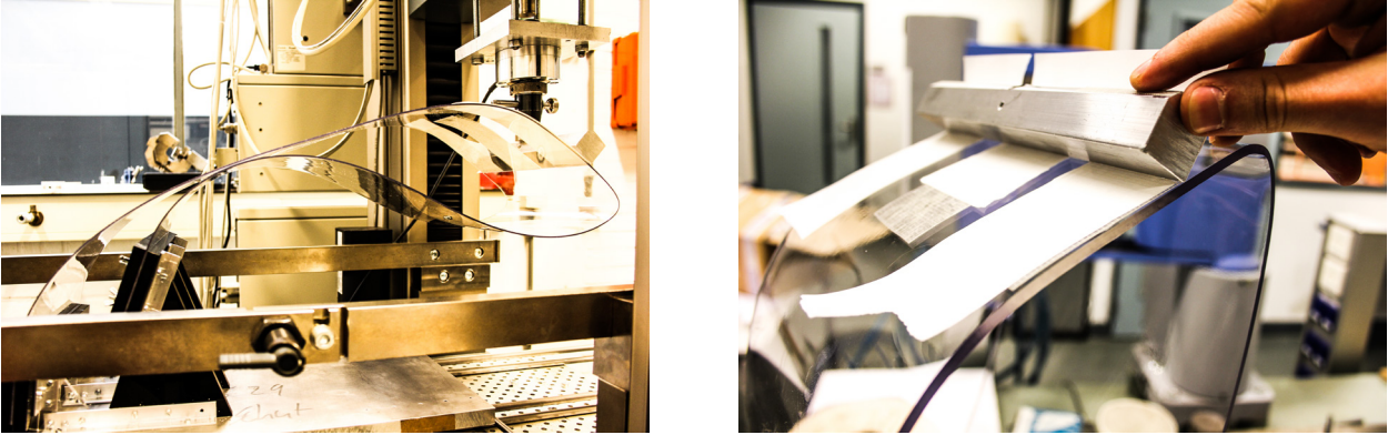
Figure C1.2: The deformed configuration (left) and the knife edge that is used to apply the vertical displacement (right). The knife edge is kept in its place due to double-sided tape.
