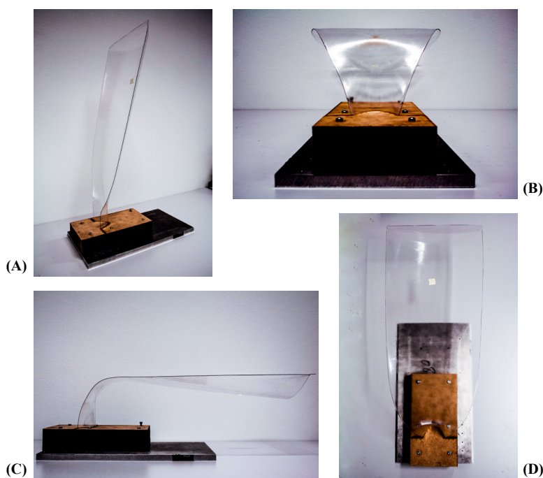
Figure P2.21: The physical model. The material is PET-G plastic. (A) presents the model in its initial and erected state. (B) illustrates a front view of the structure in its deformed state. (C) presents the structure in its deformed state. It is also noticeable that the structure is in a stable position and it does not require any external force or weight to stay in that position. (D) illustrates a top view of the deformed state.
