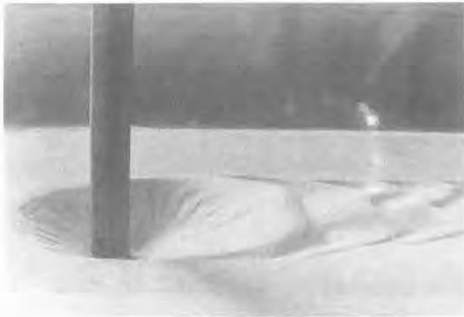
**Figure 50c.** Scour pattern 2–3 hours after test commencement [15].
