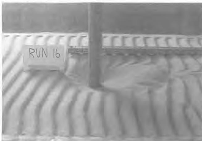
**Figure 50h.** Scour pattern due to random waves and current—Run 16.  $h = 1.167$  ft (0.36 m);  $U_c = 0.485$  ft/sec (0.148 mps);  $U = 0.508$  ft/sec (0.155 mps); wave spectrum—Jonswap ( $T = 10$  sec);  $H_{1/3} = 0.1550$  ft (0.047 m);  $D = 0.125$  ft (0.038 m);  $S_d = 0.155$  ft (0.047 m) [15].
