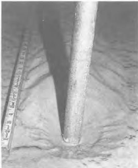
**Figure 50d.** Typical scour cavity due to a steady current  $h = 1.67$  ft (0.36 m);  $U_c = 0.485$  fps (0.148 mps);  $D = 0.125$  ft;  $S_d = 0.14$  ft (0.043 m) [15].
