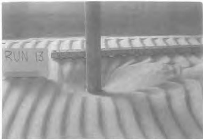
**Figure 50e.** Scour pattern due to random waves and current—Run 13.  $h = 1.167$  ft (0.36 m);  $U_c = 0.485$  fps (0.148 mps);  $U = 0.498$  ft/sec (0.1518 mps); wave spectrum—Darbyshire;  $H_{1/3} = 0.1724$  ft (0.053 m);  $D = 0.125$  ft (0.038 m);  $S_d = 0.143$  ft (0.044 m) [15].
