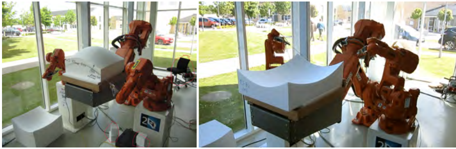
Figure 3.15: Tri-robot hot-blade cutting configuration
