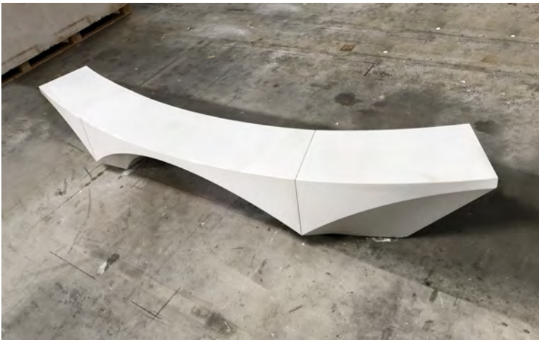
Figure 4.5: Production UPHC prototype of bench B5 for the Science Museum, Winton Gallery of Mathematics, design Zaha Hadid Computation and Design Group.
