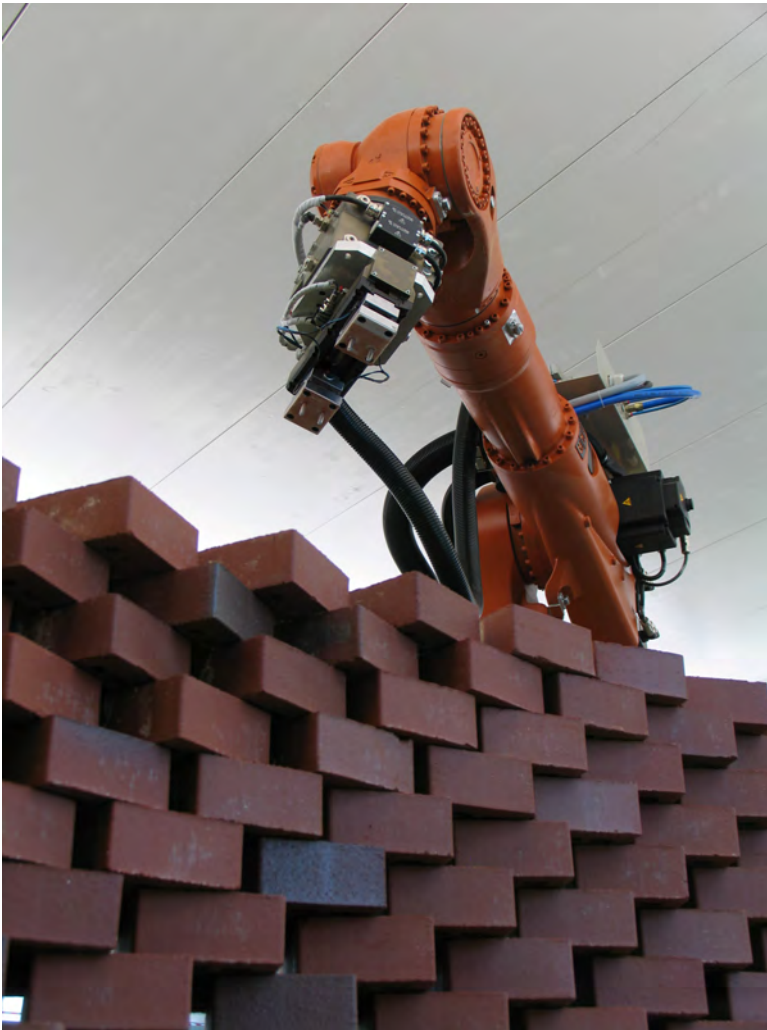
Figure 2.10: Programmed robot building up the brick wall, Gramazio & Kohler, ETH Zürich
