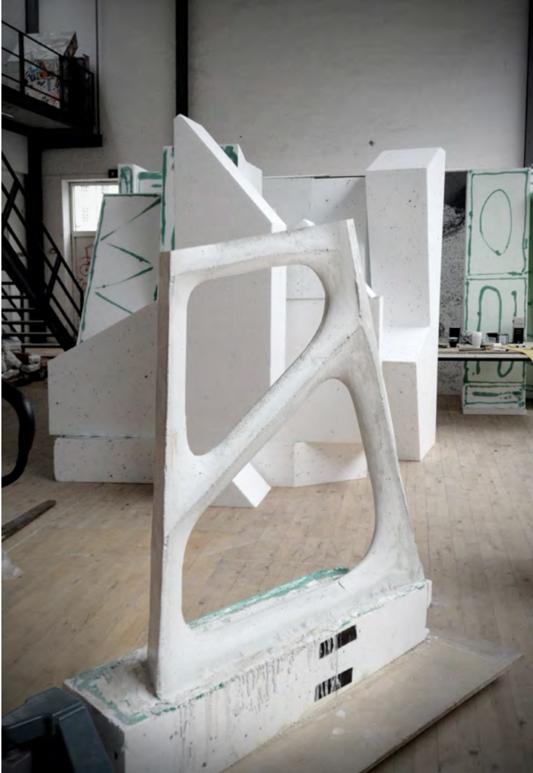
Figure 2.48: Opticut 1 : 1 sample cast, testing the casting quality of two adjacent, doubly ruled cells
