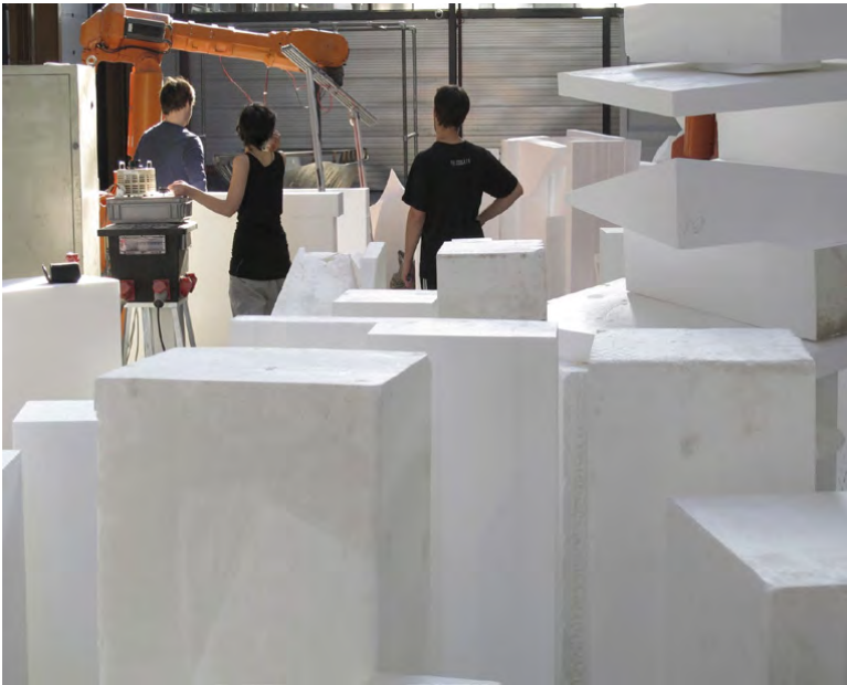
Figure 3.20: Ongoing production of the OptiCut formwork
