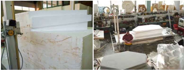
Figure 3.1: Komplot Mechanics's adapted hotwire cutting machine. Extra portal built to allow cutting both longitudinally and laterally
