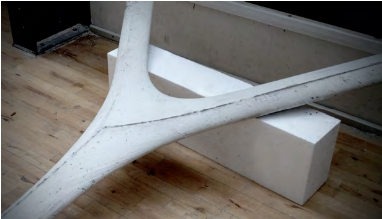
Figure 2.50: Y-joint sample cast constructed from three intersecting hyperbolic paraboloidal surfaces and six single-ruled extrusions
