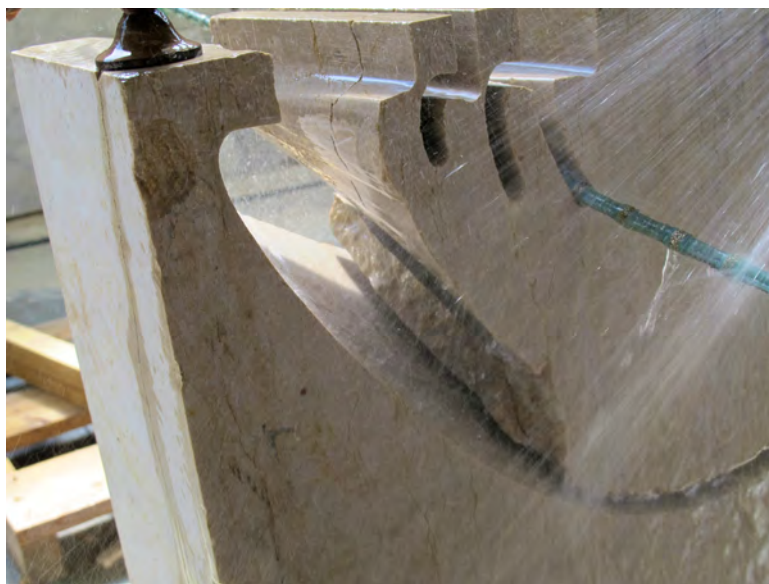
Figure 2.44: Experimental diamond wire saw setup
