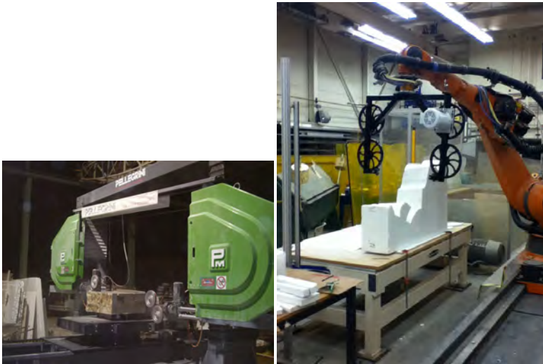
Figure 2.33: 6 axis CNC diamond wire saw (left); Wire sawing end-effector developed at the University of Michigan Taubman College (right)
