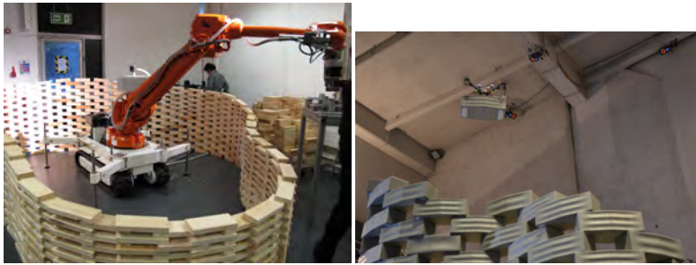
Figure 2.18: Remote sensing applied in the work of Gramazio & Kohler, ETH Zürich. (Left) Robust assembly by integrating computer vision at FABRICATE 2011. (Right) Flight assembly exposition opening at FRAC Centre, Orléans
