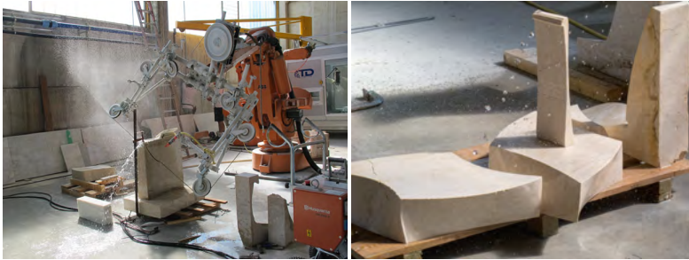
Figure 3.5: Robotic abrasive wire-saw cutting of marble blocks at Carrara, Italy (left); cut samples (right)
