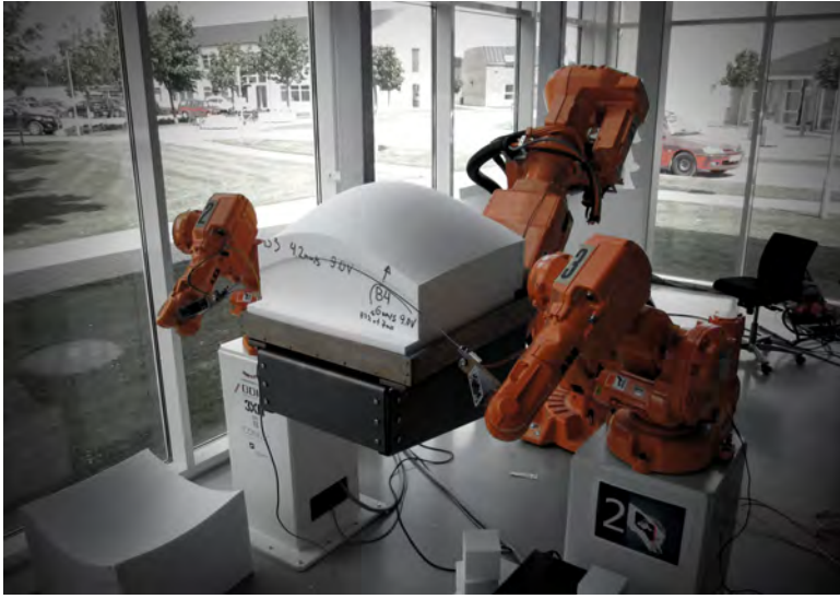
Figure 4.8: Experimental multi-robot cell deploying 3 ABB multi-move manipulators for production of doubly-curved geometries via sweeping of a flexible, heated blade along a surface.
