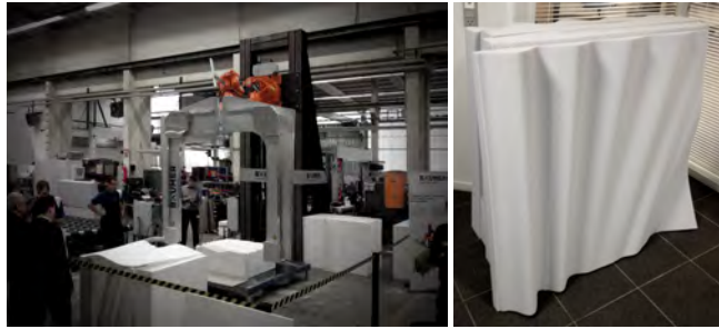
Figure 3.6: Sample geometry cut in nonflammable acoustic foam under 16 s (left) Second abrasive prototype tool, developed in collaboration with Bäumer AG (right)
