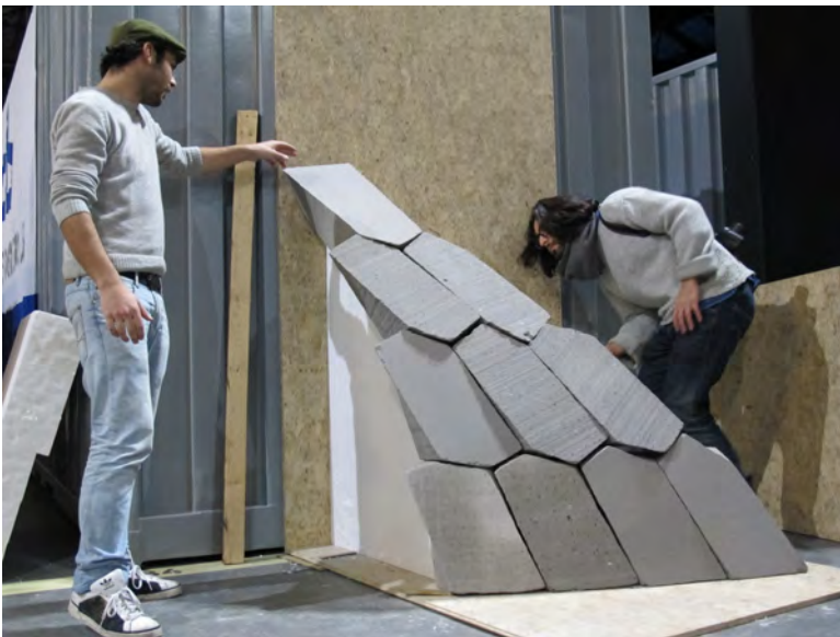
Figure 2.43: Initial test cuts in engineered limestone
