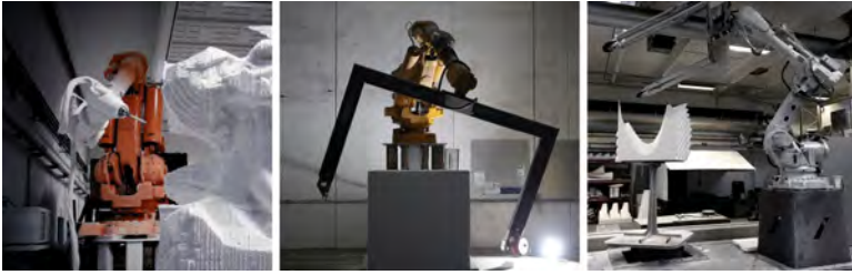
Figure 3.25: Top row, from left: Workstation 1, robotic CNC milling. Workstation 2, robotic hot-wire cutting. Workstation 3, robotic abrasive wire cutting. Bottom row: the corresponding machining result of sample 1 from each process
