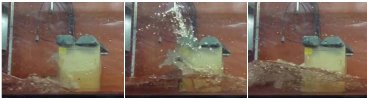
Fig. 4-1 Snapshots of physical experiment (Jansen 2019) – initial impact, deflection & reflection, quasi-steady
