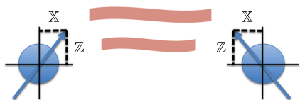
(b) Illustration showing an electron spin whose \mathbb{Z} and \mathbb{X} components are respectively correlated to the \mathbb{Z} and \mathbb{X} components of another electron spin, i.e., a quantum memory.
