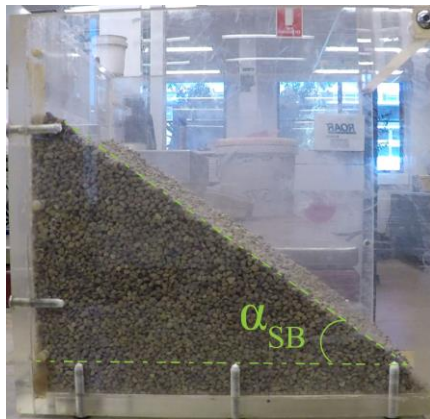
Figure 3.4 Shear angle in the shear box test
