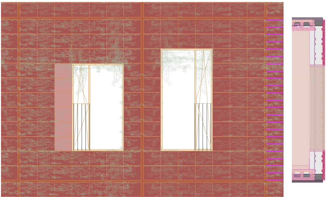
Figure 18 - Northern façade with cross-section revealing indications of interior step risers on exterior terracotta elements
