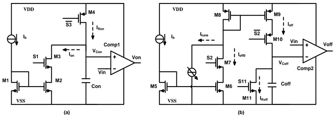
Figure 4-11: Circuit implementation of the on-time and off-time generators.
