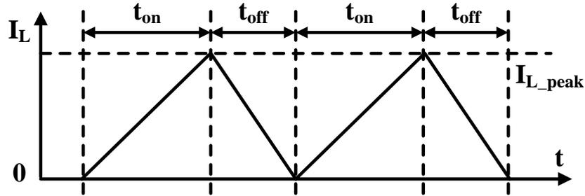
Figure 2-9: Waveform of the inductor current for the boost converter working in the boundary of CCM and DCM.
