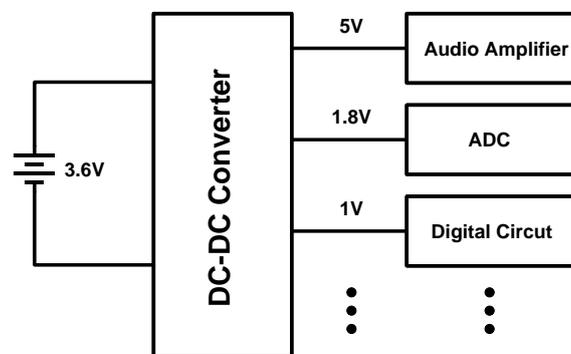
Figure 1-4: General application of a DC-DC converter in portable devices.
