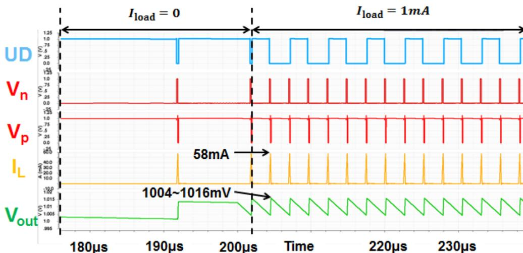
Figure 6-6: Waveforms of the boost DC-DC converter ( $I_{load} = 1mA$ ).
