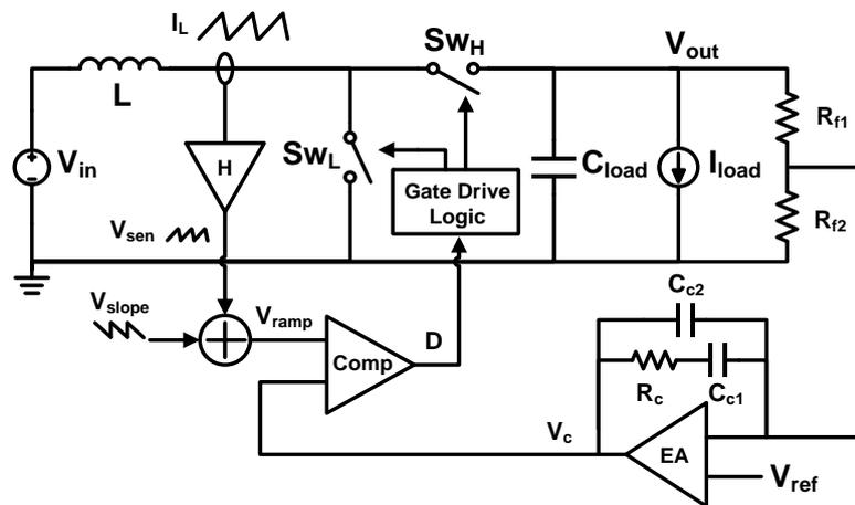
Figure 3-4: Boost DC-DC converter with a typical CCM CMC control.
