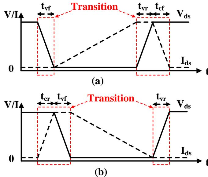
Figure 2-10: Switching waveforms of the transistor
