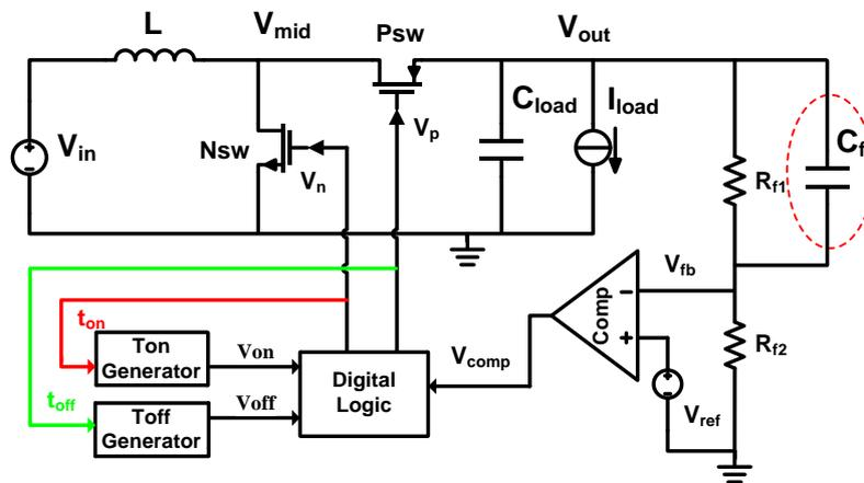
Figure 3-16: Boost DC-DC converter system with the filter cap
