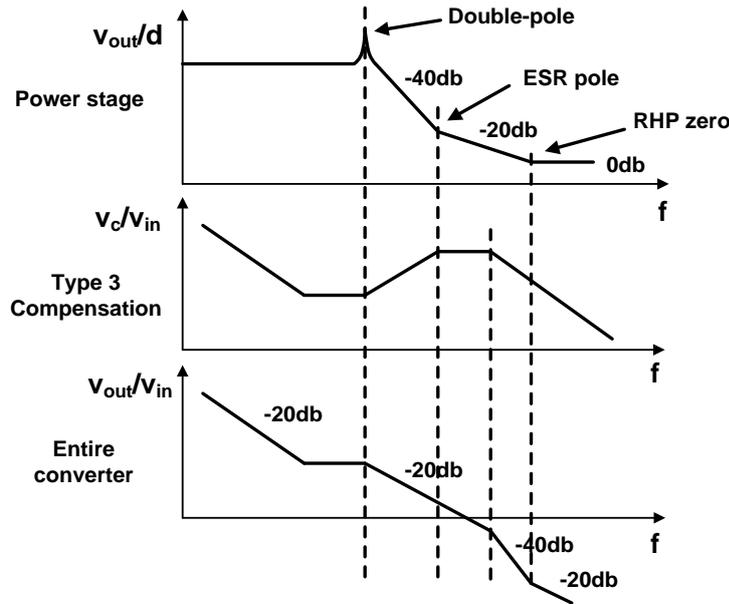
Figure 3-3: Compensation for the loop stability of a VMC boost DC-DC converter.
