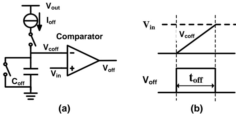
Figure 3-22: Off-time generator and its working principle.
