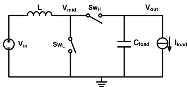
Figure 2-1: Basic Inductor-based boost DC-DC converter.
