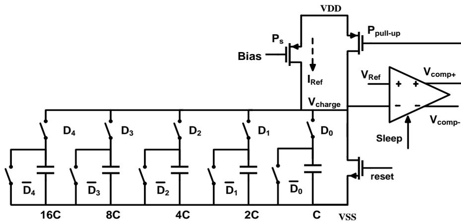
Figure 3-19: I-C time generator with DAC and sleep mode control [21].
