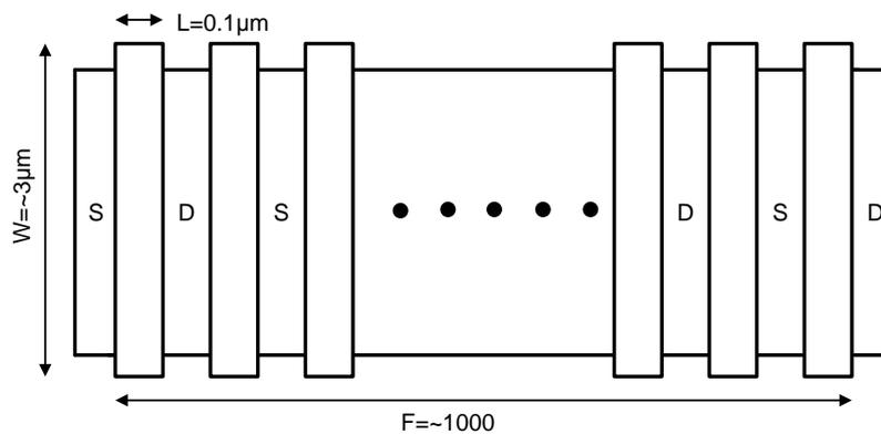
Figure 5-4: Transistor with a smaller  $W/L$  in the finger structure.
