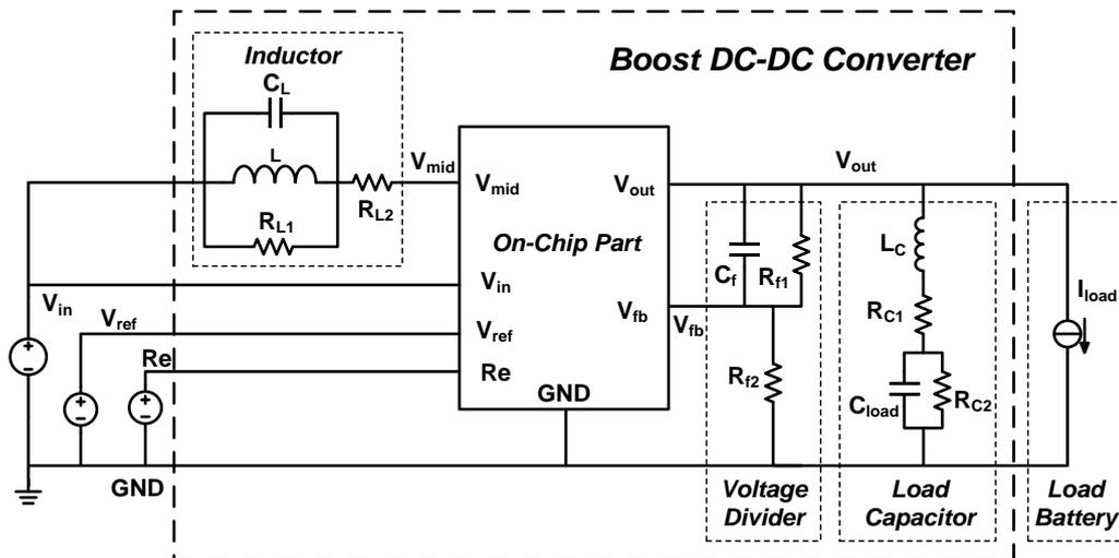
Figure 6-1: The schematic of the test bench.
