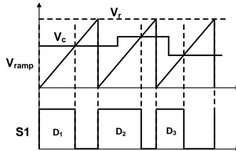
Figure 3-2: PWM signal generation by the PWM comparator.
