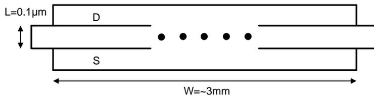
Figure 5-3: Transistor with a large  $W/L$  in the simplest structure.
