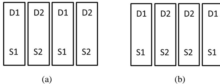
Figure 5-12: General layout techniques for current mirrors.
