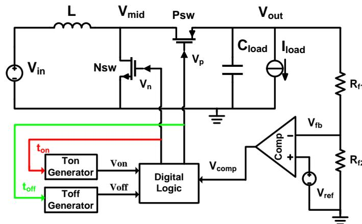
Figure 3-13: Boost DC-DC converter with an enhanced COOT control.
