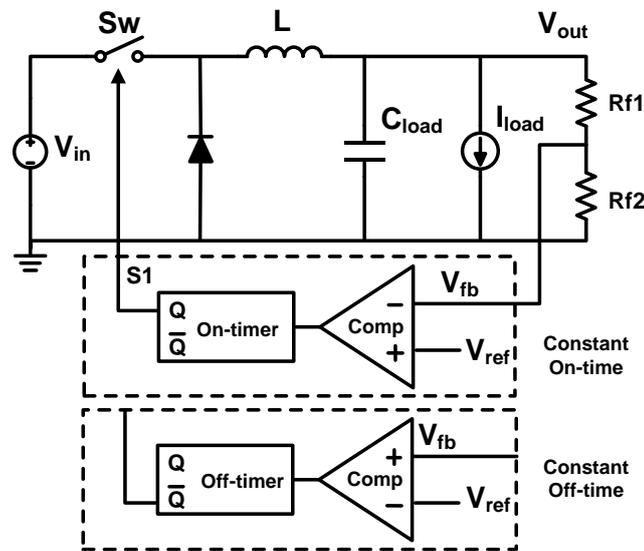
Figure 3-11: Buck DC-DC converter with COOT control [1].
