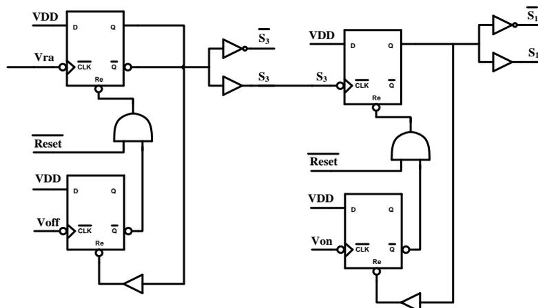
Figure 4-9:  $S_1$  and  $S_3$  generating circuits.
