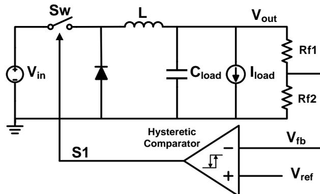
Figure 3-9: Buck DC-DC converter with hysteretic control [1].
