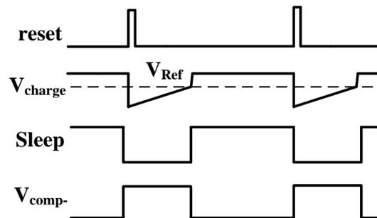
Figure 3-20: Timing diagram of main signals in the time generator [21].
