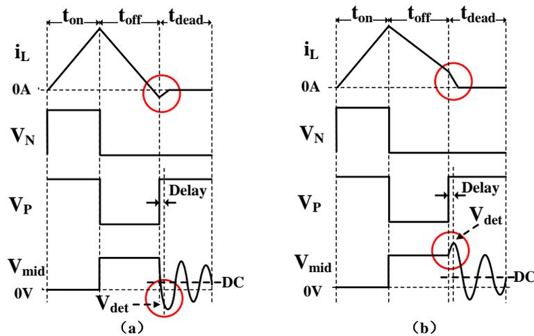
Figure 4-17: Voltage detection for an overlong or insufficient off-time.
