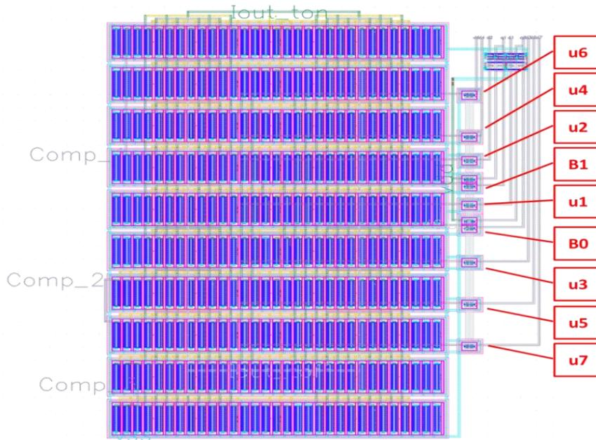
Figure 5-14: General layout techniques for current mirrors.
