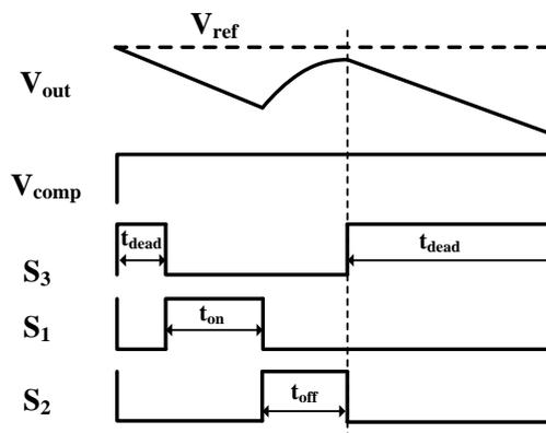
Figure 4-5: First failure mechanism of the control system.
