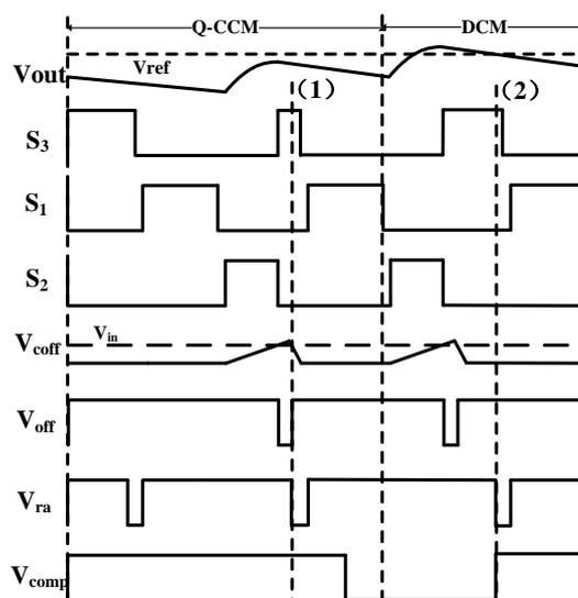
Figure 4-7: Timing diagram of quasi-CCM and DCM.
