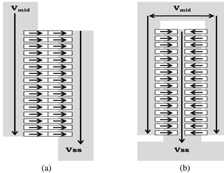
Figure 5-10: Two topologies of the NMOS power switch transistor's layout.
