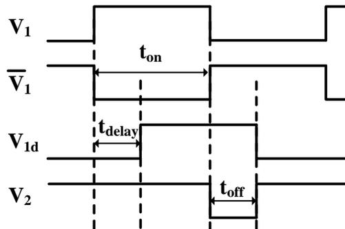
Figure 3-18: Timing diagram of main signals in the time generator. [14]
