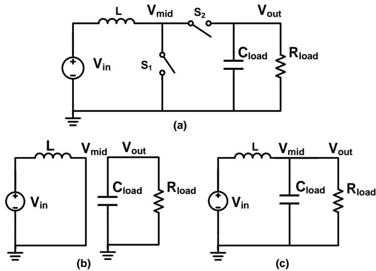
Figure 1-7: Schematic of an inductor-based boost DC-DC converter [13].
