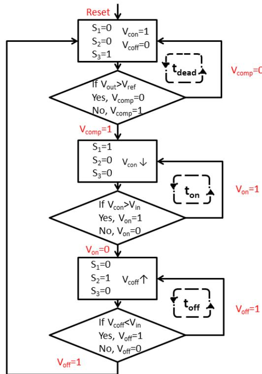
Figure 4-2: Operation flow chart of the boost DC-DC converter.
