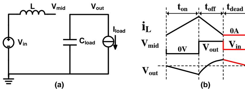
Figure 2-5: Boost DC-DC converter in the dead-time phase.
