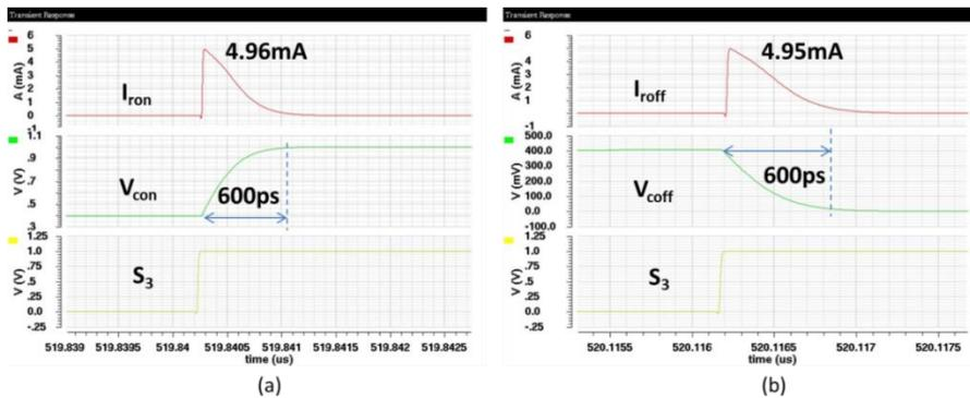
Figure 4-15: Reset of nodes  $V_{con}$  and  $V_{coff}$  in the dead-time phase.
