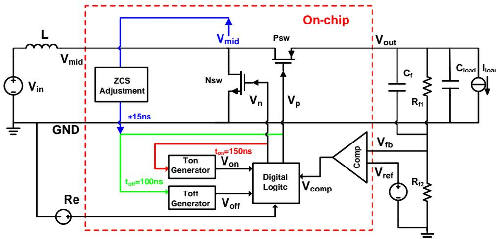
Figure 5-1: On-chip and off-chip parts of the boost DC-DC converter.
