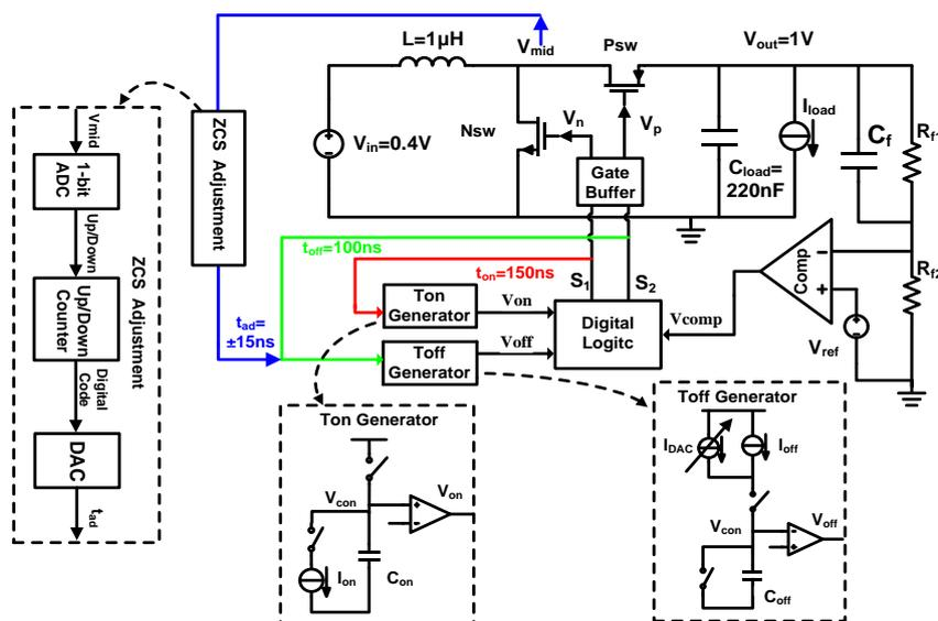
Figure 4-1: Entire boost DC-DC converter system designed in this work.
