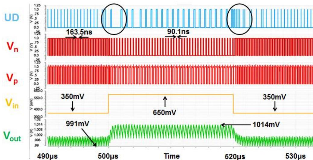
Figure 6-9: Responses of the boost converter to an input voltage variation.
