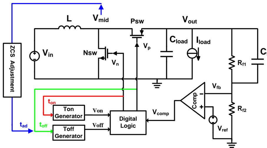
Figure 3-25: Entire boost DC-DC converter with AOOT control and ZCS adjustment.
