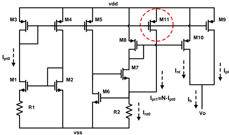
Figure 4-26: Final schematic of the reference current generator.
