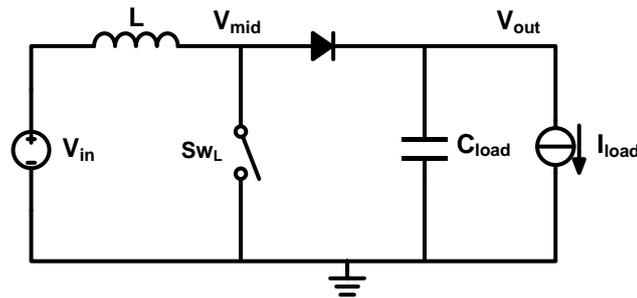
Figure 2-7: Asynchronous boost DC-DC converter.
