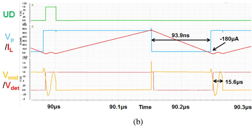
Figure 6-5: Verification of the ZCS adjustment technique ( $I_{load} = 10mA$ ).
