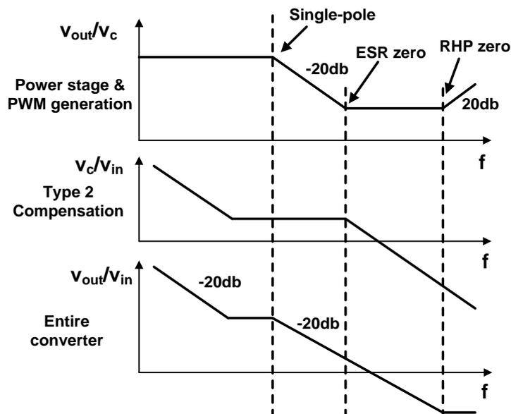
Figure 3-5: Compensation for the loop stability of a CMC boost DC-DC converter.
