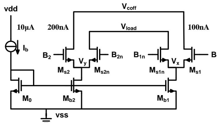
Figure 4-20: Two current branches controlled by 2-bit binary digital code in the DAC.
