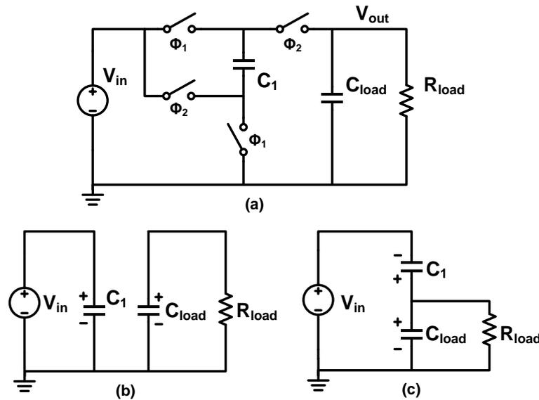
Figure 1-6: Schematic of a charge-pump DC-DC converter [13].
