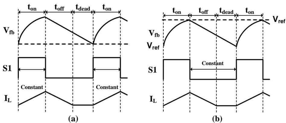
Figure 3-12: Timing diagram of the buck converter with
