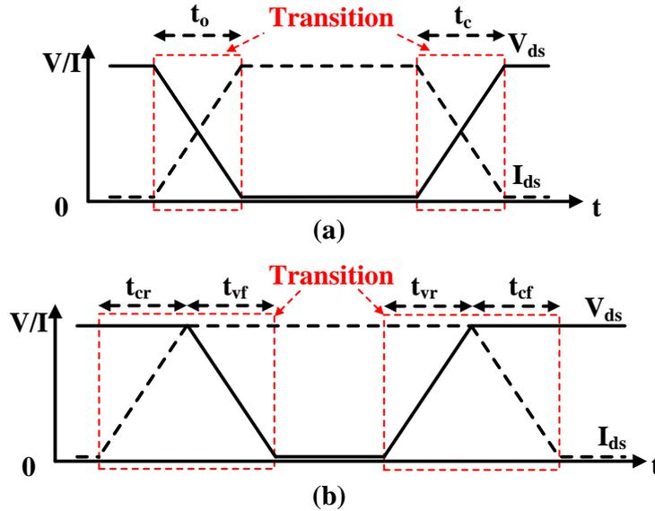
Figure 2-8: Switching waveforms of the transistor
