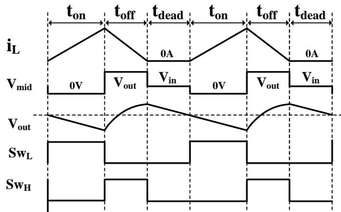
Figure 2-6: Timing diagram of the main signals in a DCM boost converter.
