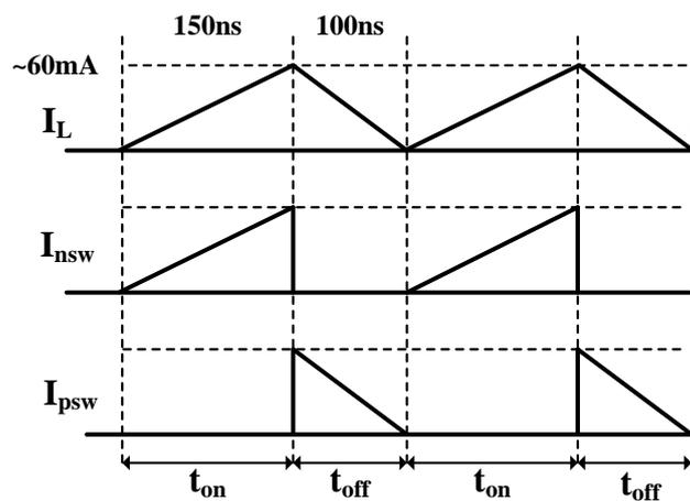
Figure 5-7: Currents flowing through the inductor and power switch transistors.
