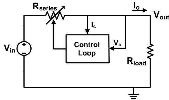
Figure 1-5: Schematic of a linear voltage converter [13].
