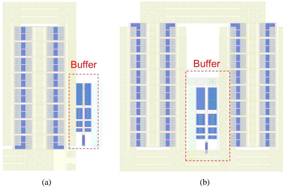
Figure 5-11: Final layout of the NMOS (a) and PMOS (b) power switches with buffers.
