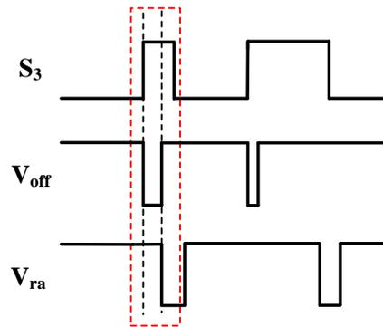
Figure 4-8: Timing diagram of  $S_3$  triggering and resetting.
