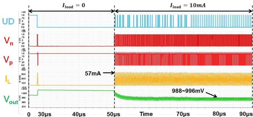
Figure 6-3: Waveforms of the boost DC-DC converter ( $I_{load} = 10mA$ ).
