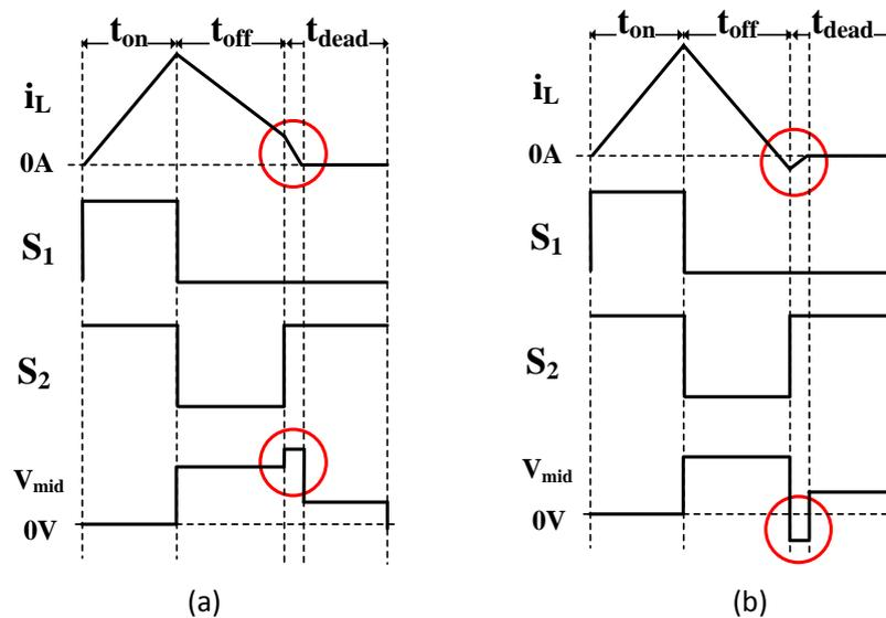
Figure 3-23: Boost converter with overly short off-time (a) and overly long off-time (b)
