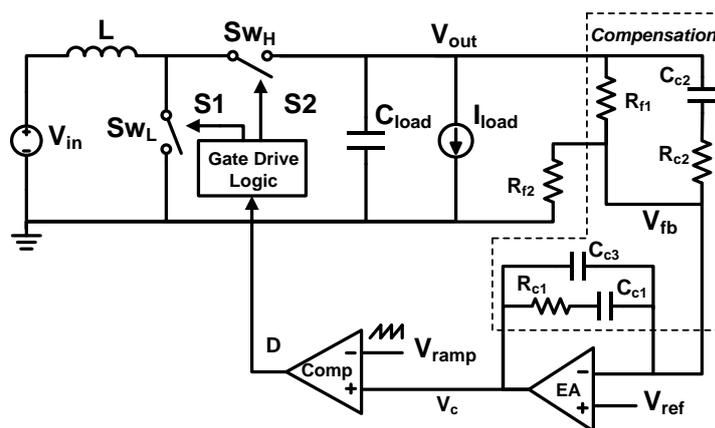
Figure 3-1: Boost DC-DC converter with a typical CCM VMC control.
