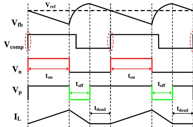
Figure 3-14: Timing diagram of the boost converter with an enhanced COOT control.
