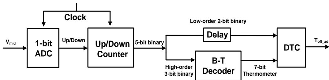
Figure 4-19: System-level diagram of the ZCS adjustment block
