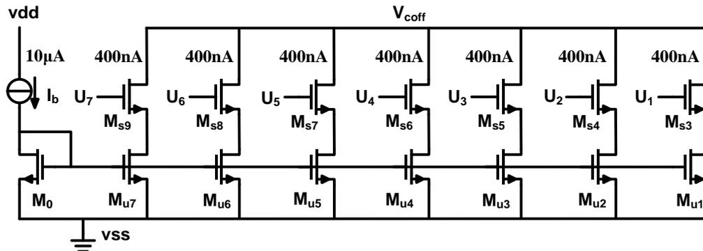
Figure 4-21: Seven current branches controlled by 7-bit unary digital code in the DAC.
