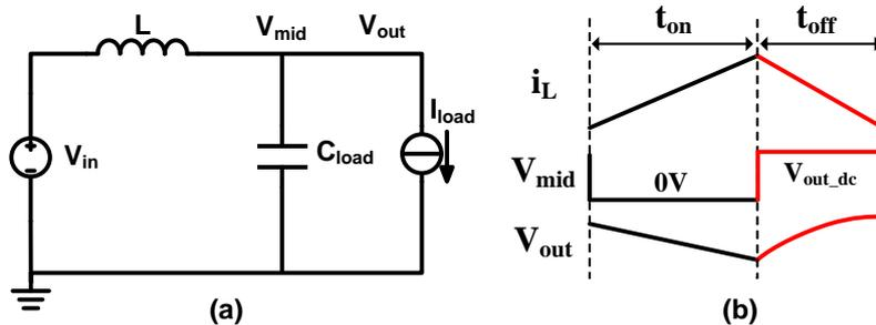
Figure 2-3: Boost DC-DC converter in the off-time phase.
