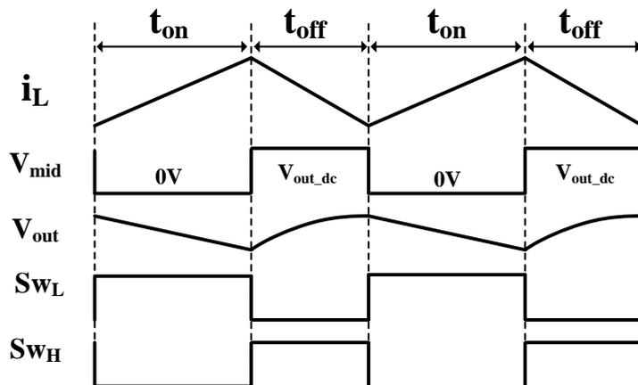
Figure 2-4: Timing diagram of main signals in a CCM boost converter.
