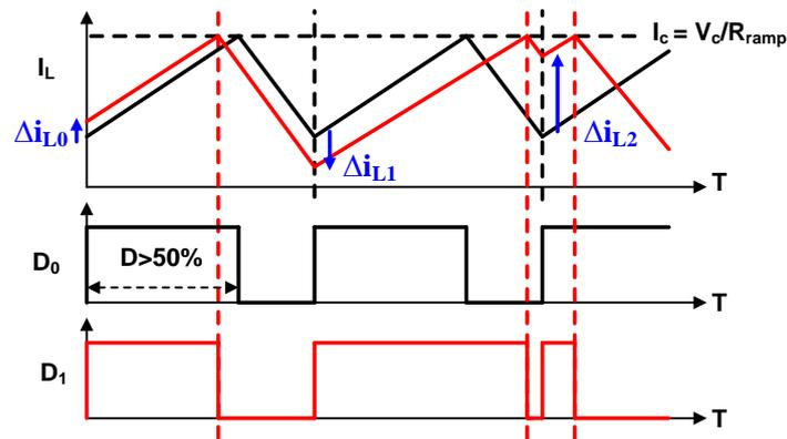
Figure 3-6: Subharmonic oscillation when duty cycle exceeds 50%.
