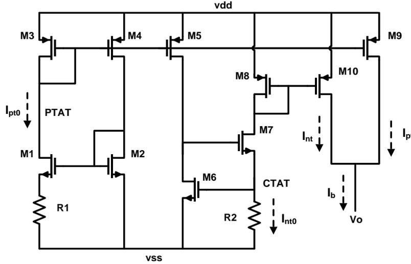
Figure 4-25: Combination of a PTAT current source and a CTAT current source [4].
