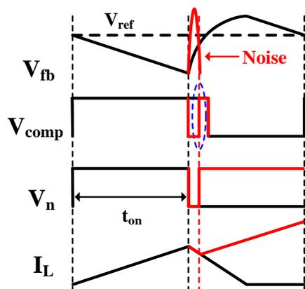
Figure 3-15: Control system is sensitivity to the noise at the node  $V_{fb}$ .
