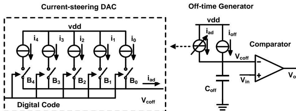
Figure 4-18: Current-mode DTC for the off-time calibration.
