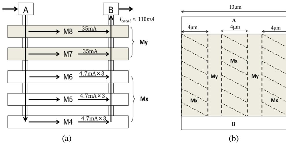
Figure 5-9: 5-layer metal wire, (a) cross-section view, (a) top view.
