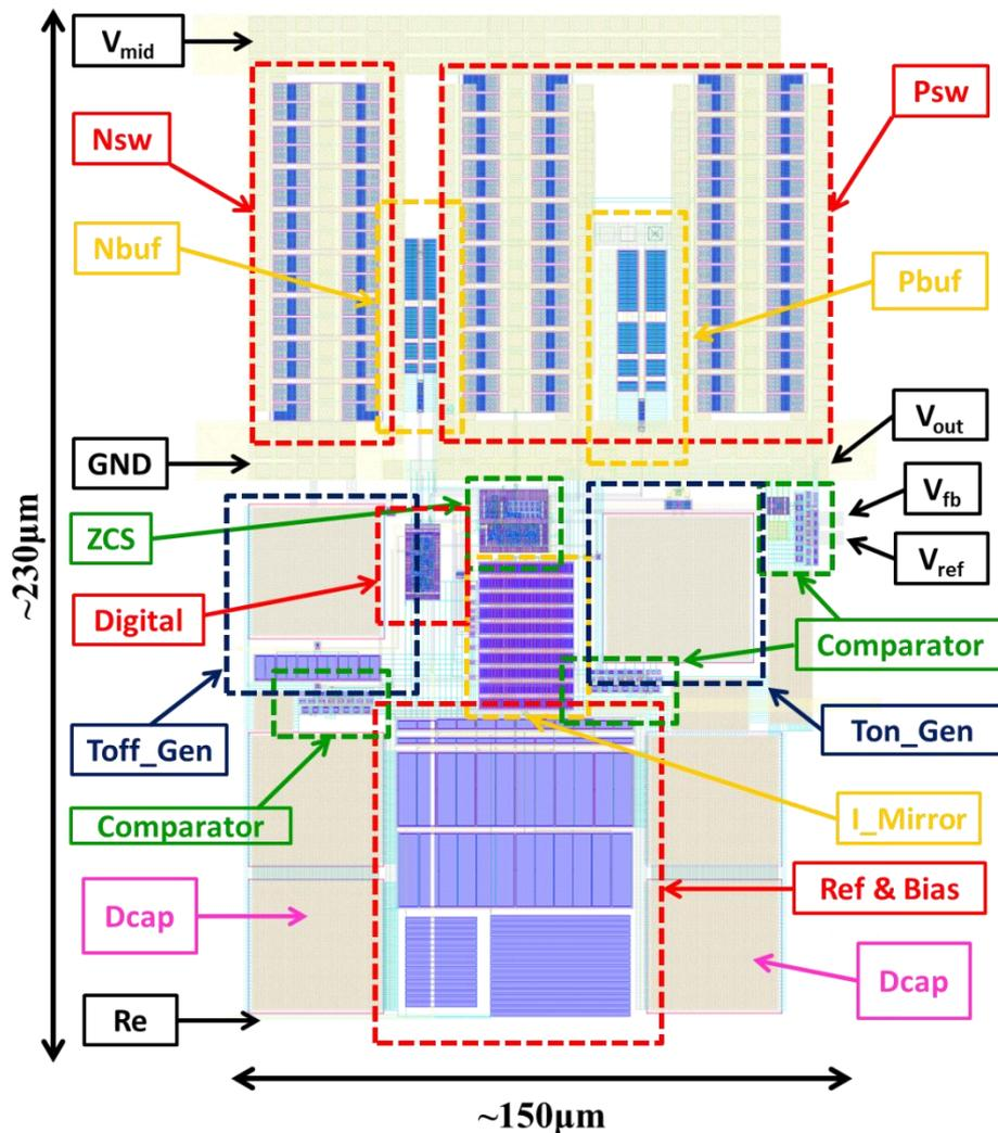
Figure 5-2: Layout of the entire on-chip part of the boost DC-DC converter.
