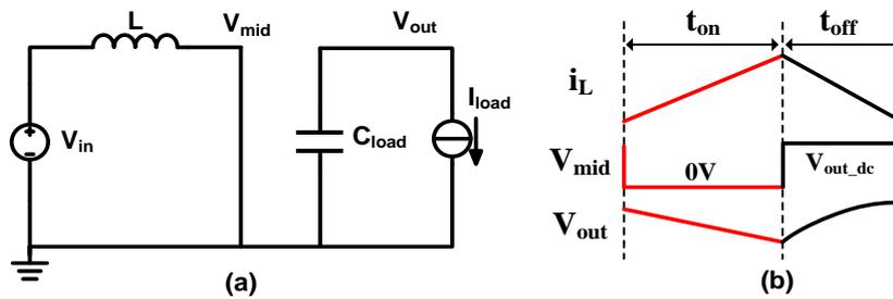
Figure 2-2: Boost DC-DC converter in the on-time phase.
