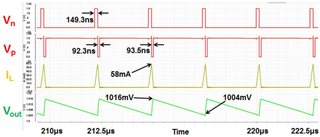
Figure 6-7: Zoom-in waveforms of the boost DC-DC converter ( $I_{load} = 1mA$ ).
