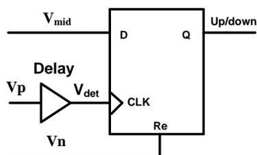
Figure 4-16: A D flip-flop 1-bit ADC.
