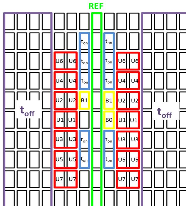
Figure 5-13: Layout topology for the current mirrors in this work.
