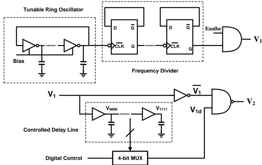
Figure 3-17: One approach to implement the time generators. [14]
