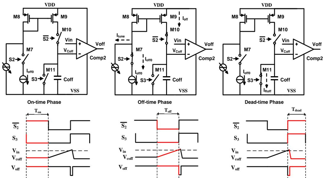
Figure 4-13: Different working phases of the off-time generator.
