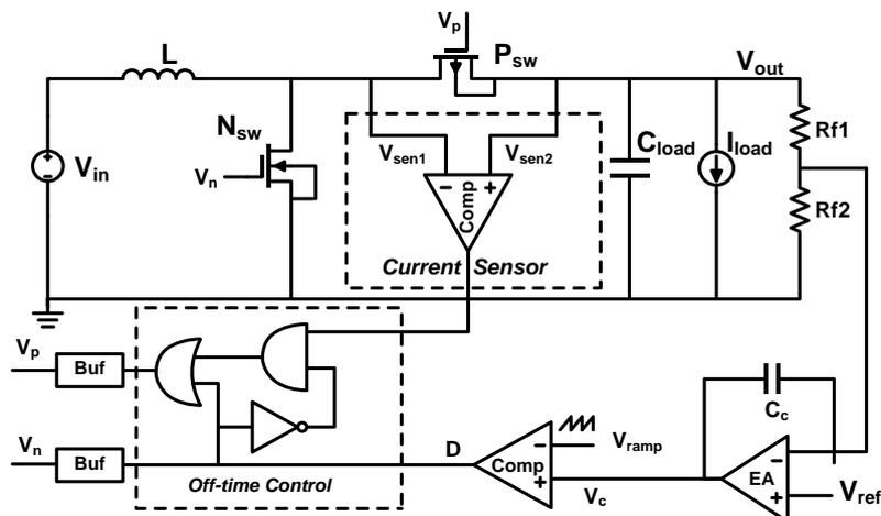
Figure 3-8: DCM VMC boost DC-DC converter system [9].
