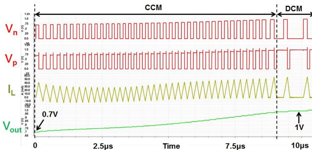
Figure 6-2: Startup phase of the boost DC-DC converter.
