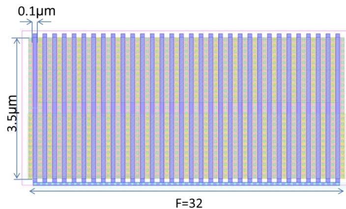
Figure 5-6: Unit cell of the power switch transistor.
