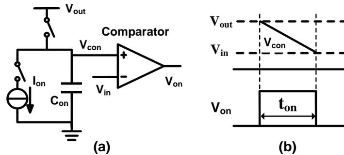
Figure 3-21: On-time generator and its working principle.
