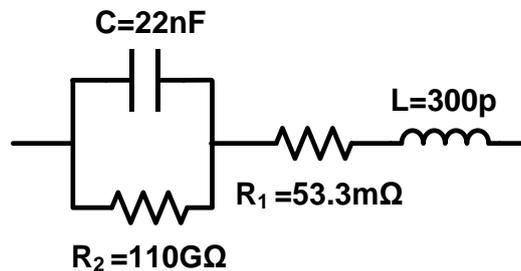
Figure 2-12: Equivalent schematic model of the capacitor “C0603JB0J223K030BC”.
