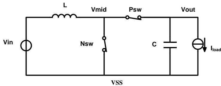
Figure 4-10: Output of the boost converter short to the ground.
