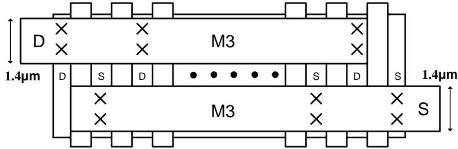
Figure 5-8: Source and drain connection of a unit transistor.
