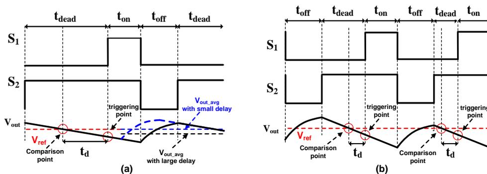
Figure 4-22: Comparator delay effect under (a) low load and (b) high load.
