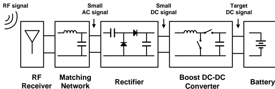
Figure 1-3: RF energy harvesting system used to charge the battery.
