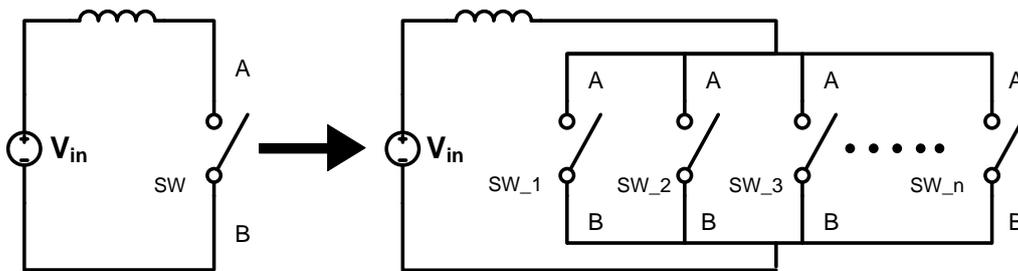
Figure 5-5: Segmentation of the large power switch transistor.
