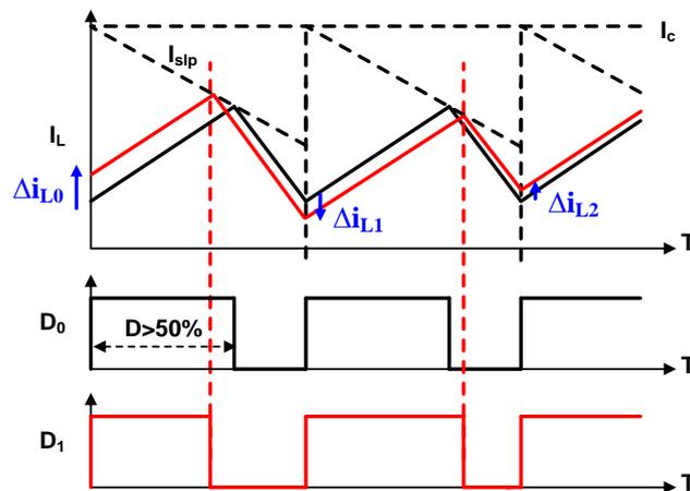
Figure 3-7: Slope compensation to eliminate the subharmonic oscillation.
