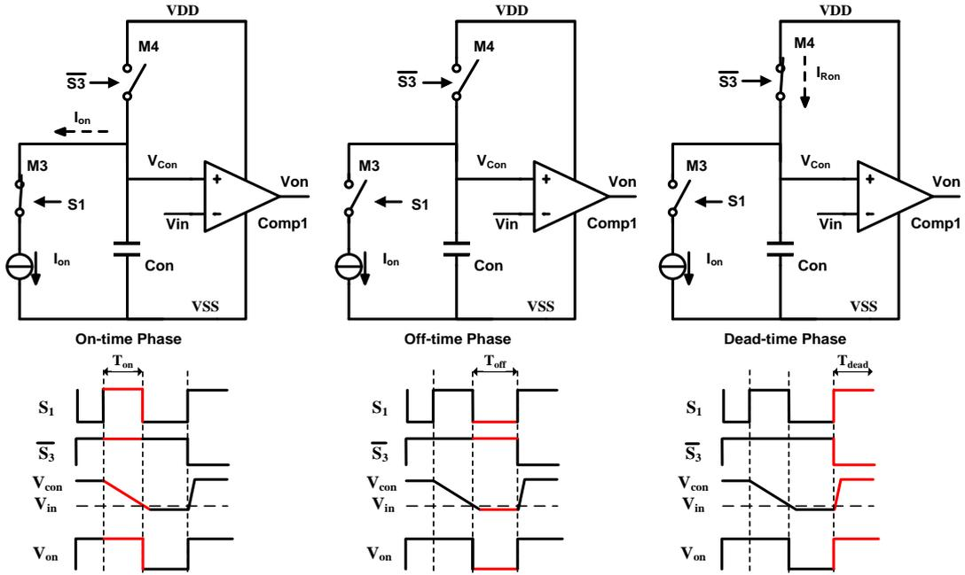
Figure 4-12: Different working phases of the on-time generator.
