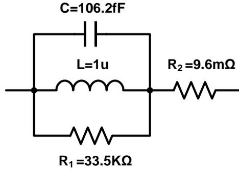
Figure 2-11: Equivalent schematic model of the inductor “CLF7045T-1R0N”.
