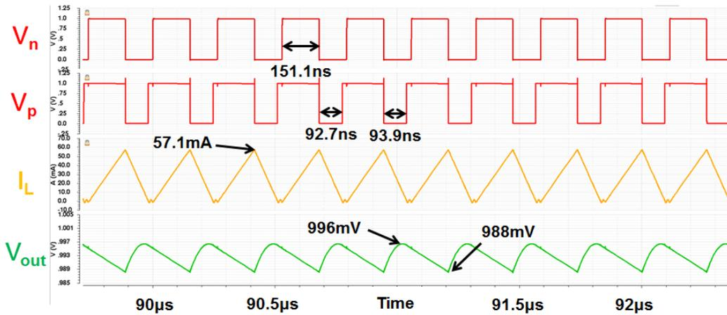
Figure 6-4: Zoom-in waveforms of the boost DC-DC converter ( $I_{load} = 10mA$ ).
