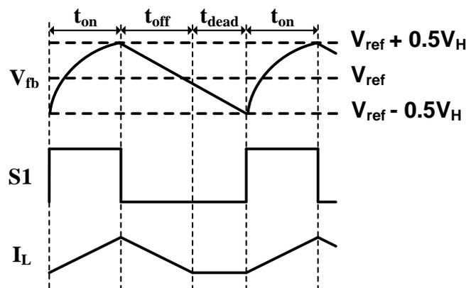
Figure 3-10: Timing diagram of the buck converter with hysteretic control.
