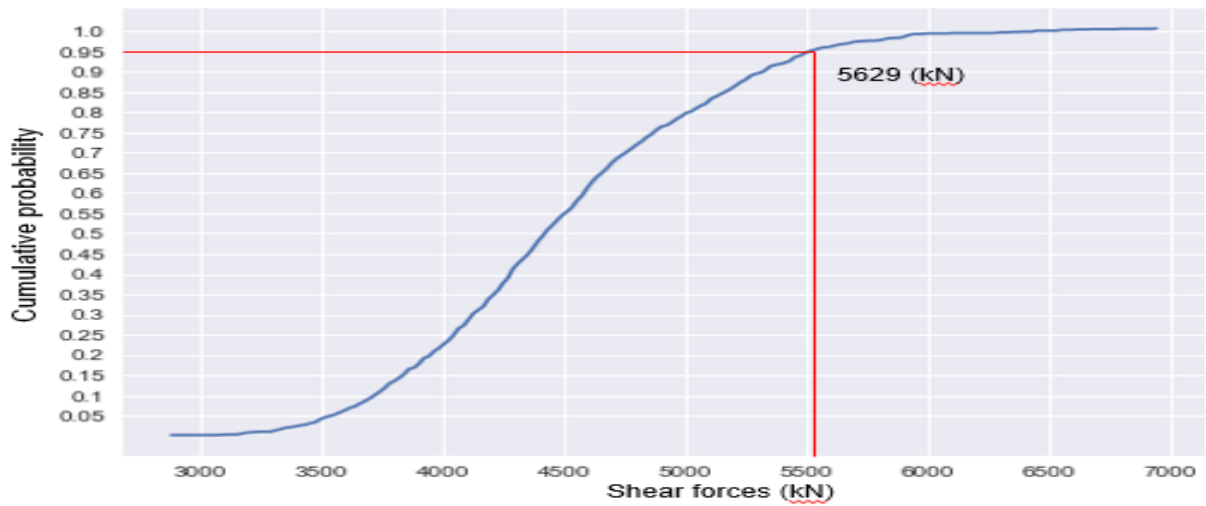
Figure 5.18 Cumulative density function plot of reliability against reduced threshold in 1 st model
