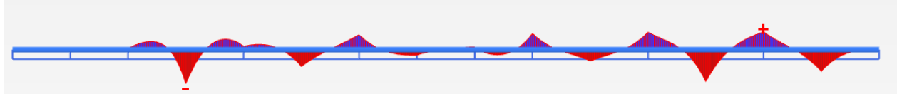
Figure 5.20 Shear force distribution along tunnel line in 1 st model from PLAXIS Output in one generation
