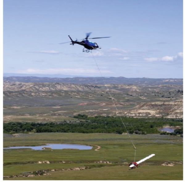
Figure 2.7: FDEM based AEM (HEM) system [18]
