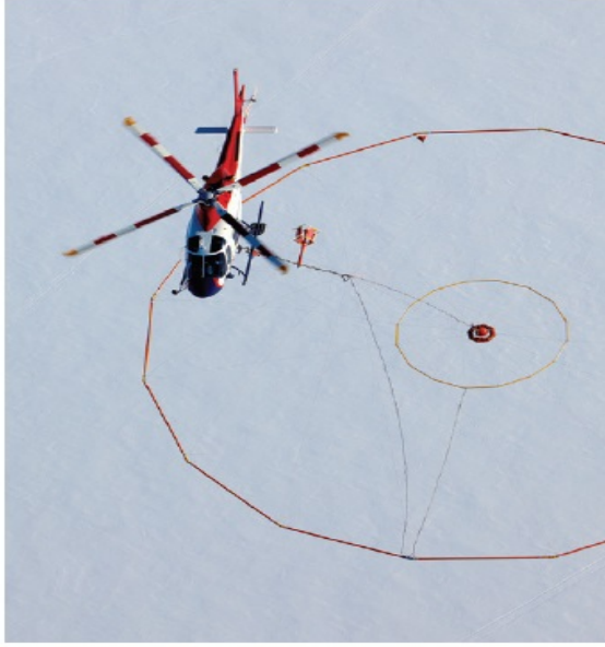
Figure 2.6: TDEM based AEM (HEM) system [17]
