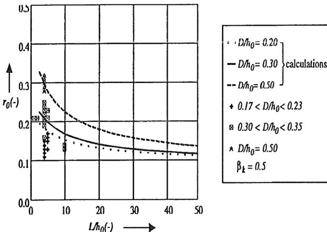
Figure 6 Relative turbulence intensity as function of  $L/h_0$  (2-D experiments; rough)
