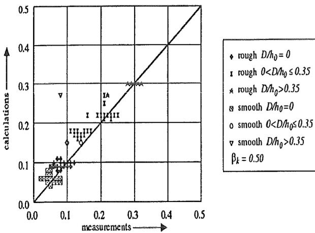
Figure 4 Relative turbulence intensity (2-D experiments)
