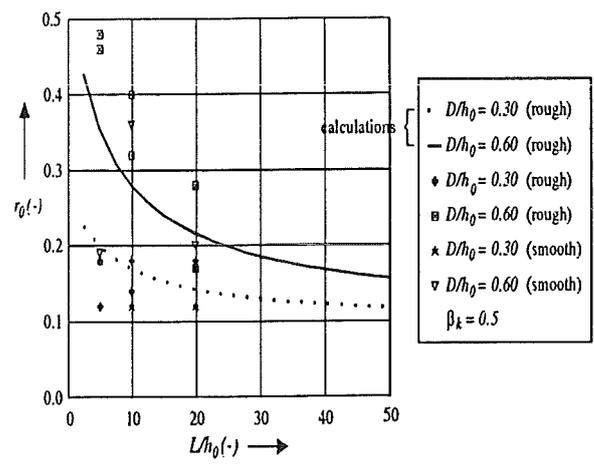
Figure 7 Relative turbulence intensity as function of  $L/h_0$  (3-D experiments)
