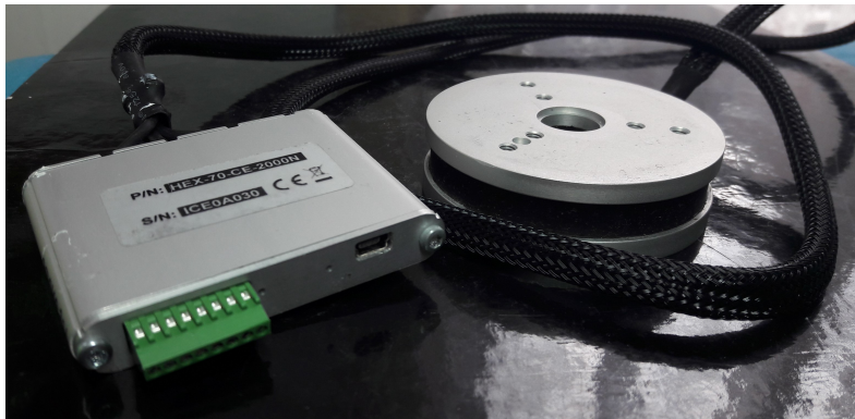
Figure 4.3: One of the 6 axis force sensors used in this study. Brand: OptoForce. Model: HEX-70-CE-2000N, interface type USB. On the right is the sensor, left is the data acquisition unit with micro USB exit port.
