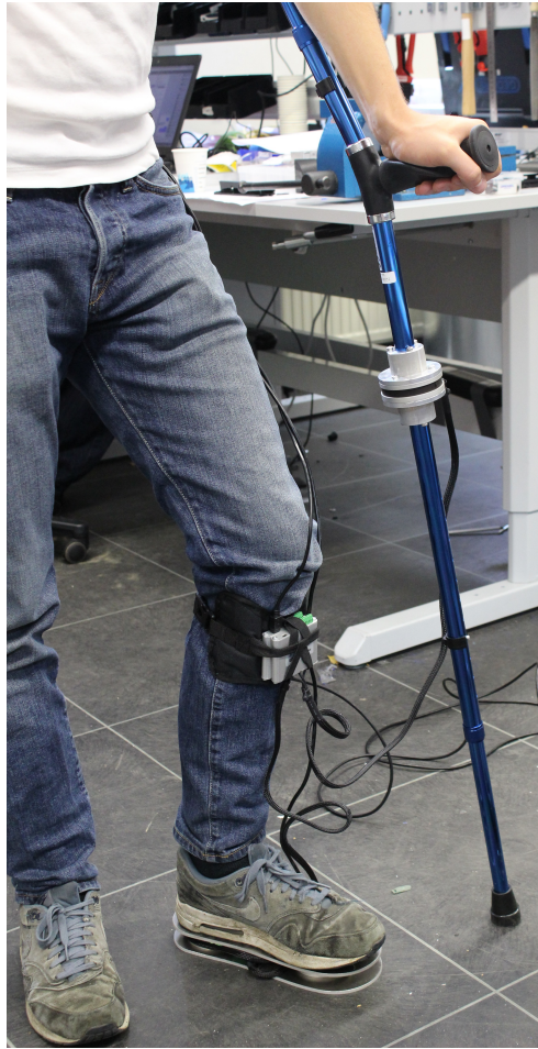
Figure 4.4: Wearable sensor shoe, crutch and DAQ unit fixture on lower leg. The straps to strap the wearable sensor shoe to the foot had not been made when this photo was taken.
