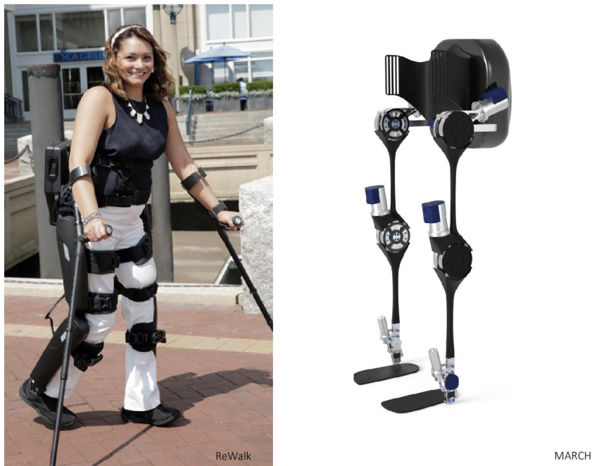
Figure 1.1: The photo on the left shows a paraplegic user in the ReWalk exoskeleton (ReWalk Robotics, www.rewalk.com ), the image on the right features a rendering of the MARCH I exoskeleton design.
