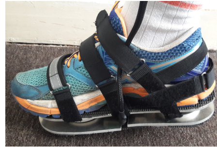
Figure 4.2: The wearable sensor shoe can be easily put on and adjusted using the black Velcro straps.
