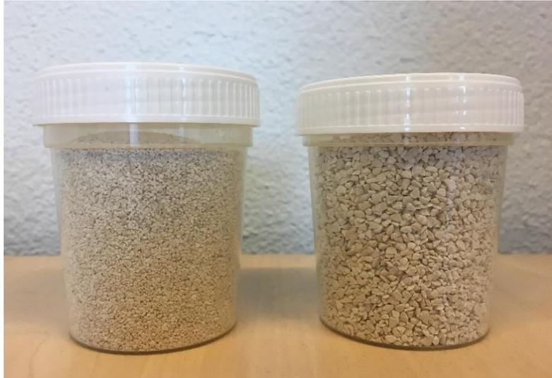
Figure 7. Filter bed material: Juraperle 0.5-1.2 mm and Juraperle 1.0-2.0 mm
