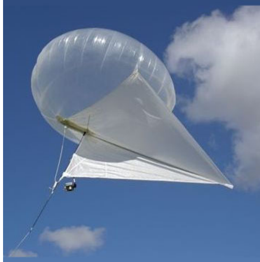
Figure 12.5: The 7.0 m 3 Helikite developed by Allsopp Helikites.
