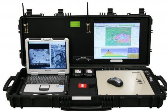
Figure 12.8: Monitoring station with an example configuration of the modular electronic compartment included.
