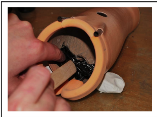
39. Apply carbon fiber material and fixate it with glue.
