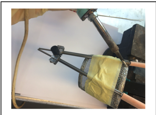
15. Solder the two guiding tubes to the small wire mesh socket.
