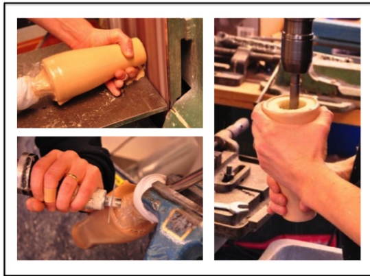
31. Remove the foam so only the socket is left.
