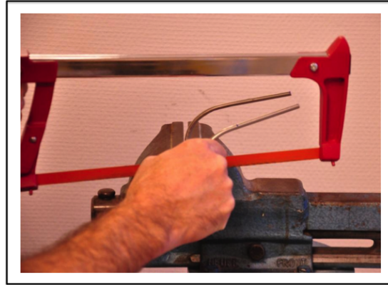
14. Saw in the middle of the condyle brace.
