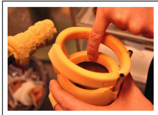
42. Check it and later coat the foam with irathane to protect against abrasion.
