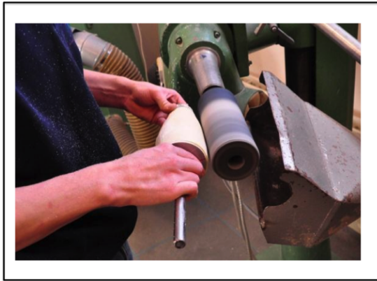
25. Customize the dummy so it fits to the patient's residual limb.
