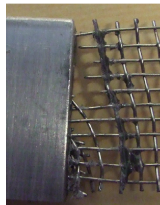
(b) Aluminium H-profile, mesh is broken instead of the glue.
