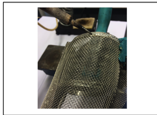
30. Solder the socket's wire mesh edges to the small socket.
