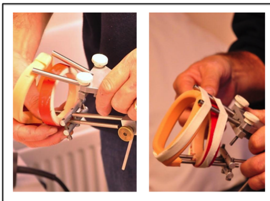
11. Monitor the test-socket-holder and fix it with adhesive tape.
