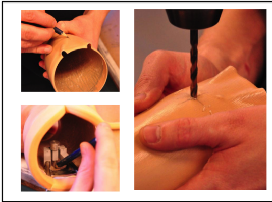
37. Mark the position of the button and drill a hole.
