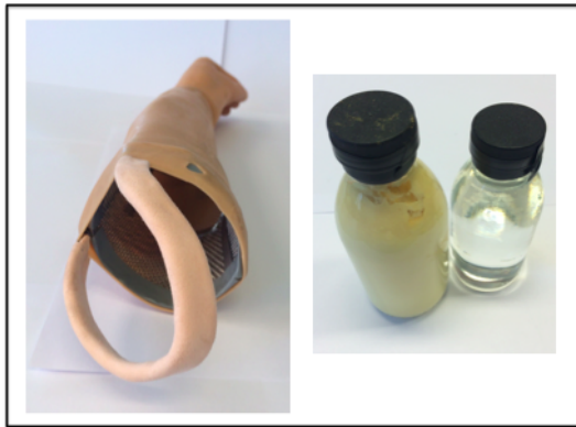
43. Coat the foam braces with with irathane to protect against abrasion.
