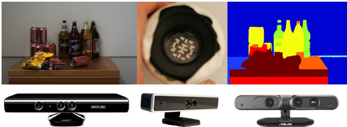
Figure 18 Upper row: example image from [30] showing an RGB scene(left), aperture coding pattern using a thin cardboard layer(center), and the resulting ‘layered’ depth map (right). Lower row: Kinect, depth Sense and Xtion.
