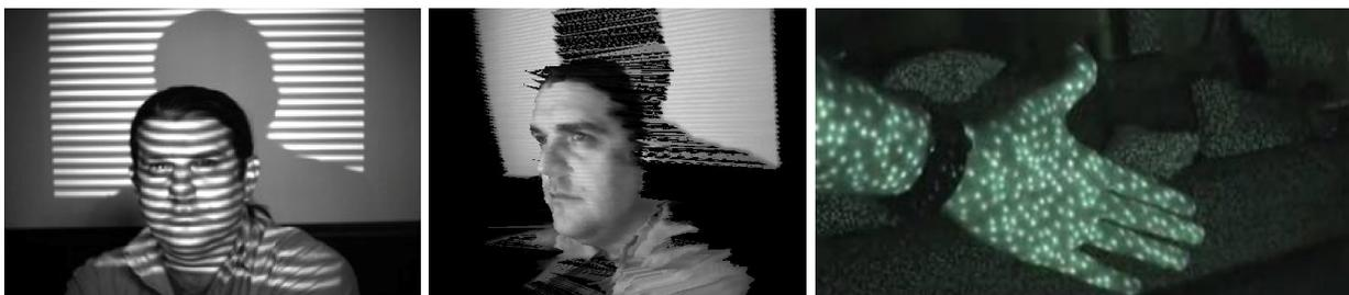
Figure 17 Person with a projection of a sinusoidal grayscale banded image (left), the result after processing (center) and an example of Kinect's speckle structure (right).
