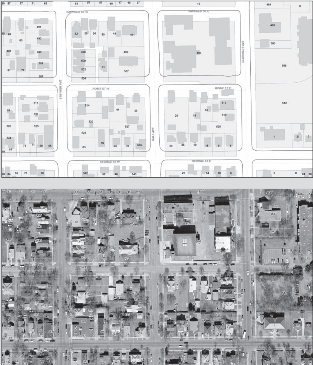
Figure 8.10 Example of poor alignment of building footprints and with parcel information, and road centreline information in Ramsey County
