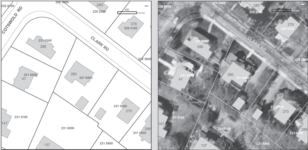
Figure 9.6 Alignment between parcel and building information (left) and building information and aerial (right) at Goddard Avenue, Town of Brookline (MA)
