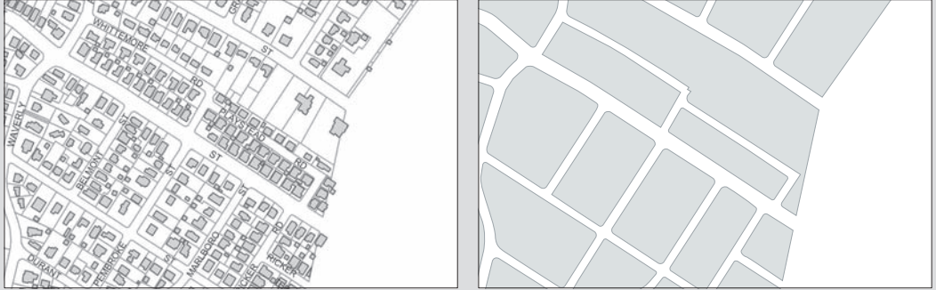
Figure 4.5 Differences in information content at similar scales (left side topographic dataset of City of Newton, MA (USA); right side road centre line of maps.google.com)
