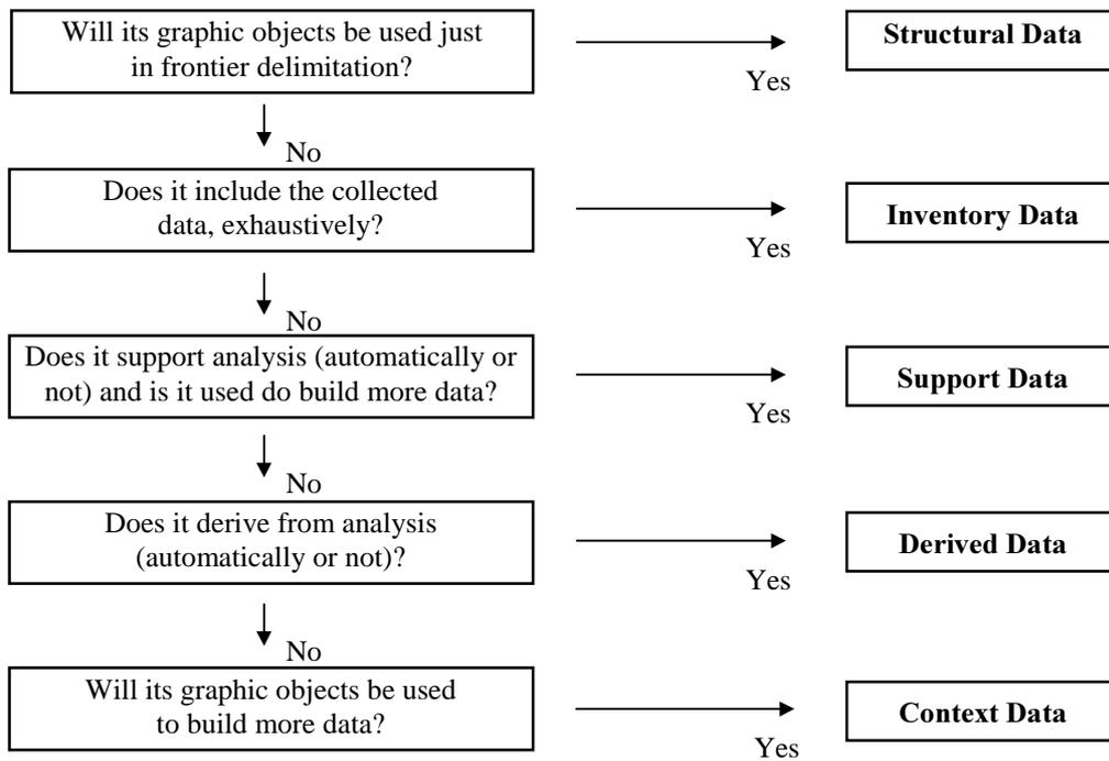
**Figure 3.1.4.7** – Classification of information according to its cartographic use
