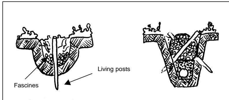
**Figure 3.3.5.3.2.3** – Scheme of a drainage by fascines
