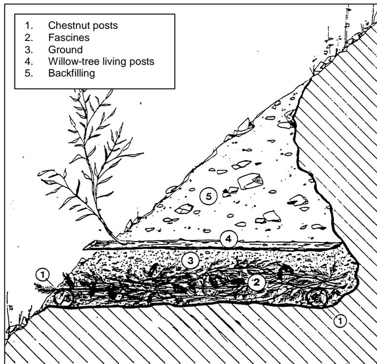
**Figure 3.3.5.3.2.5** – Scheme of a bench-terraces
