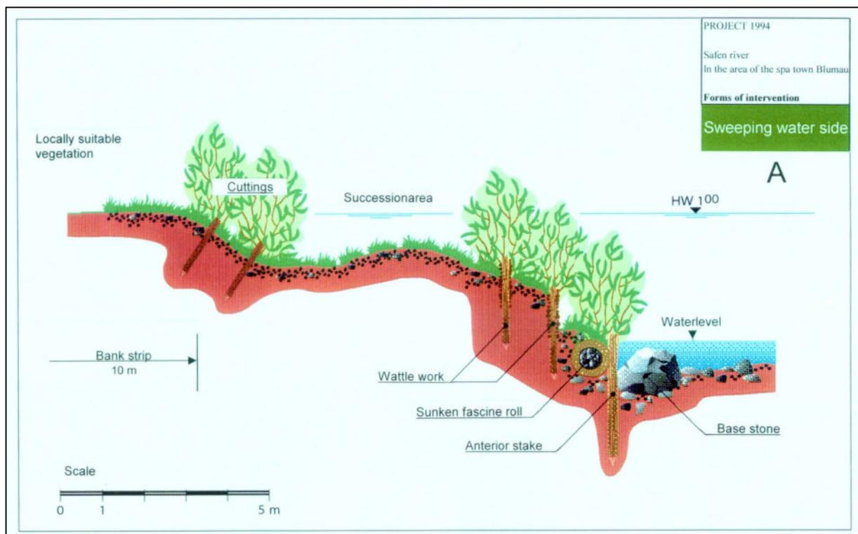
Figure 3.3.3.2.2 a - Sweeping water side (type “A” measure)
