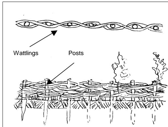
**Figure 3.3.5.3.2.4 – Scheme of wattling**
