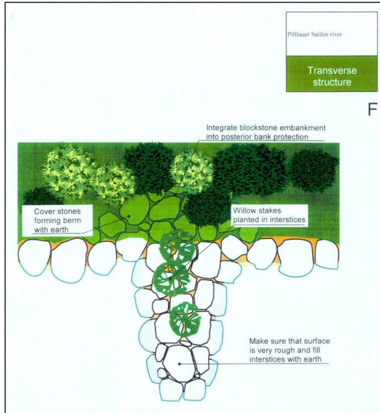
**Figure 3.3.3.2.2 f – Top view of stone groyne with cutting (type “F” measure)**
