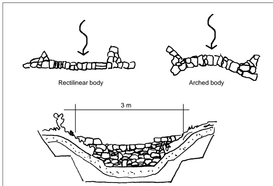
Figure 3.3.5.3.2.1 c – Scheme of a dry check dam
