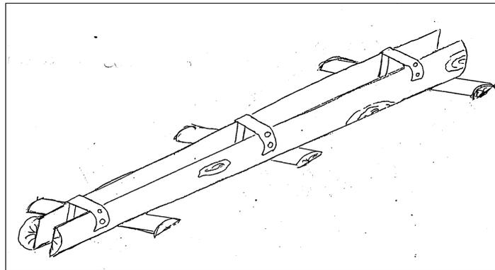
**Figure 3.3.5.3.2.8** – Scheme of a cross gutter
