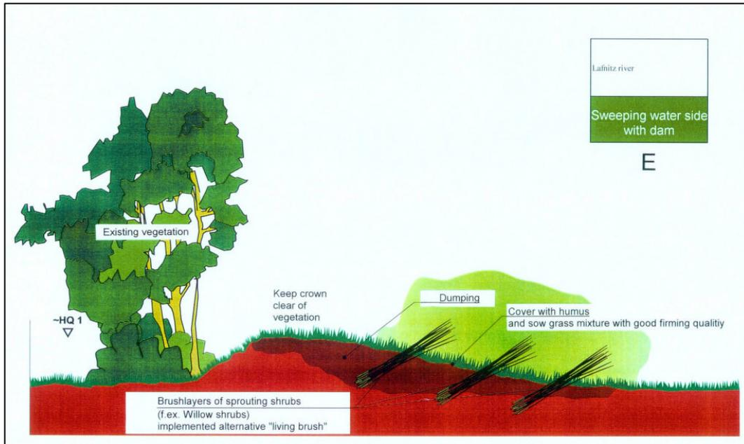
**Figure 3.3.3.2.2 e - Sweeping water side with dam along the banks (type “E” measure)**
