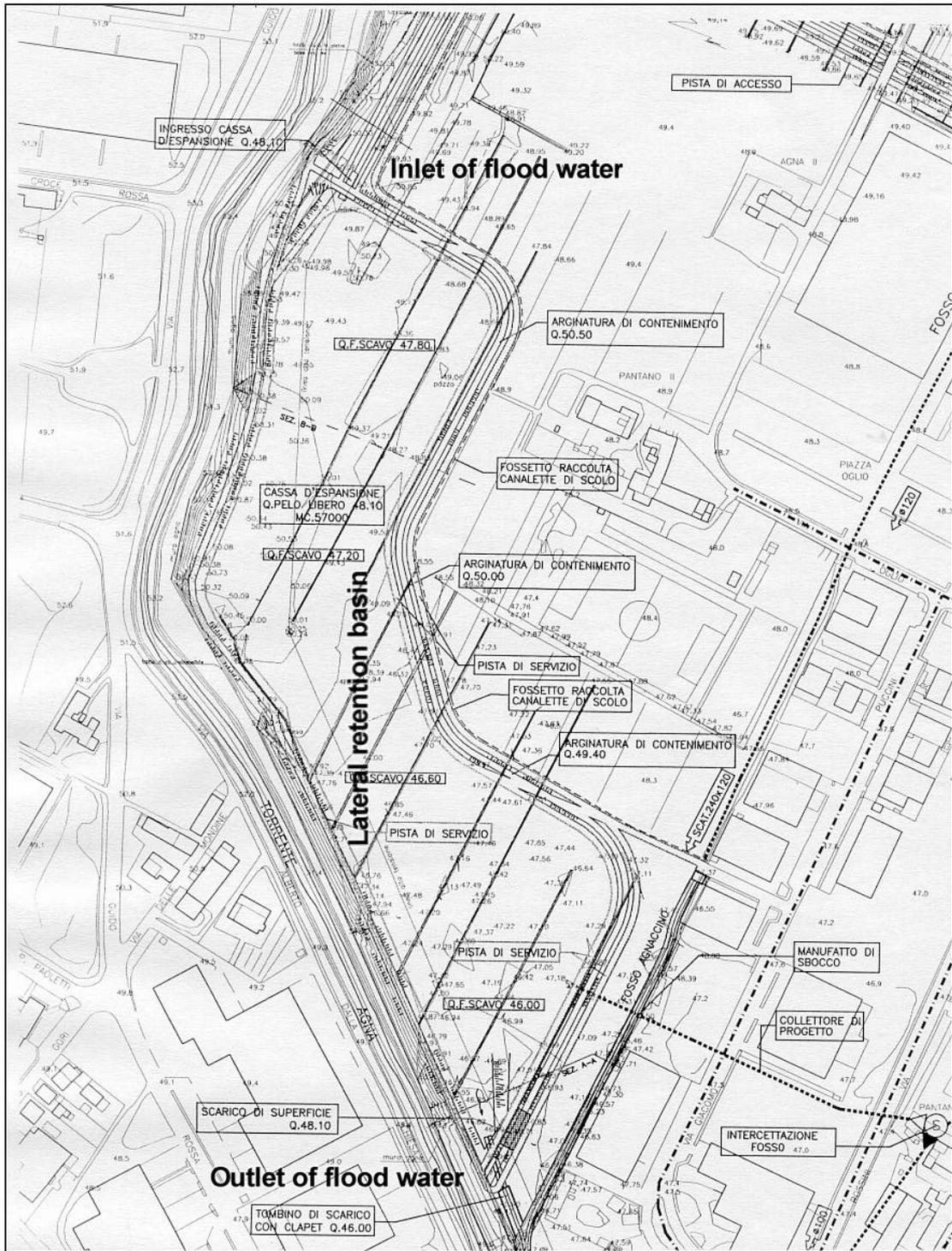
Figure 3.3.2.3 – Lateral retention basin near Prato - Italy (scale 1:4 000)
