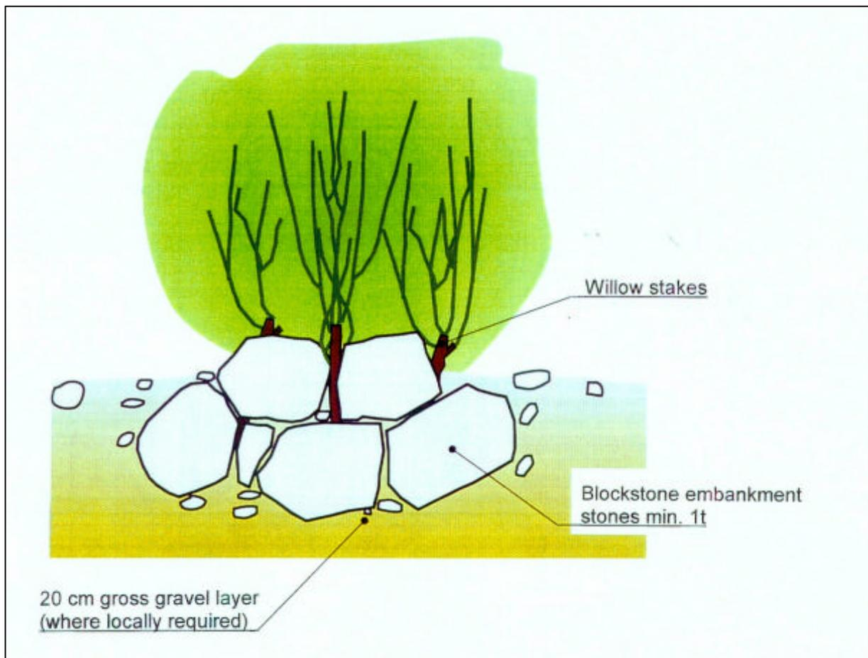
**Figure 3.3.3.2.2 f 2 –** Front view of stone groyne with cutting (type “F” measure)
