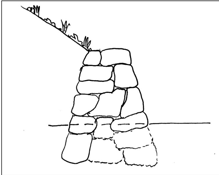
**Figure 3.3.5.3.2.6** – Scheme of a stone retaining wall
