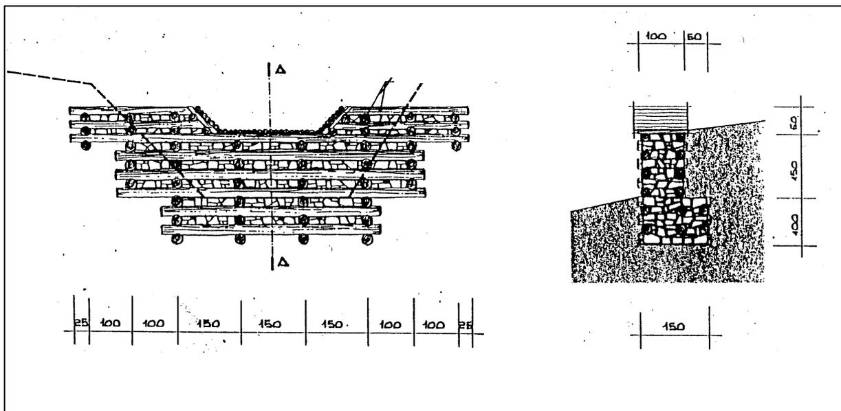
Figure 3.3.5.3.2.1 b – Scheme of a timber and loose stones check dam
