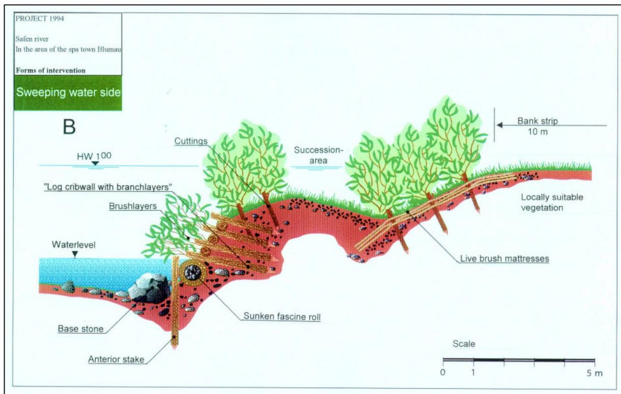
Figure 3.3.3.2.2 b - Sweeping water side (type “B” measure)
