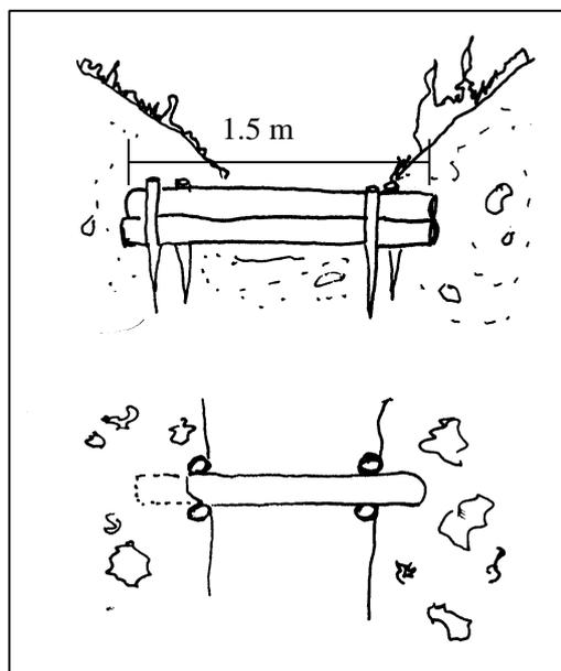
**Figure 3.3.5.3.2.1 a** – Scheme of a timber check dam
