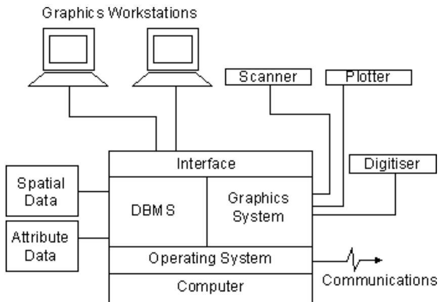
**Figure 3.1.4.1 a** – The physical components of a GIS
