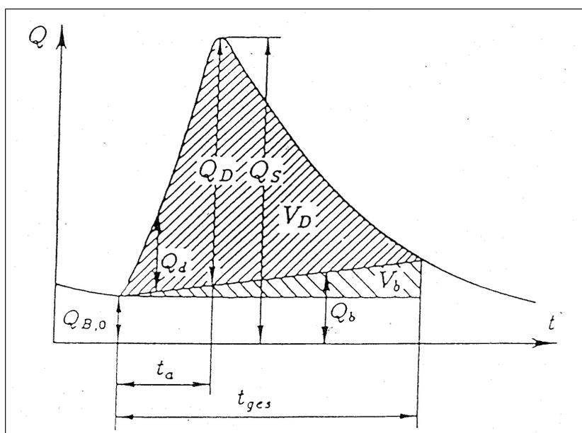
**Figure 3.3.2.2 b - Scheme of a flood event and characteristics**
