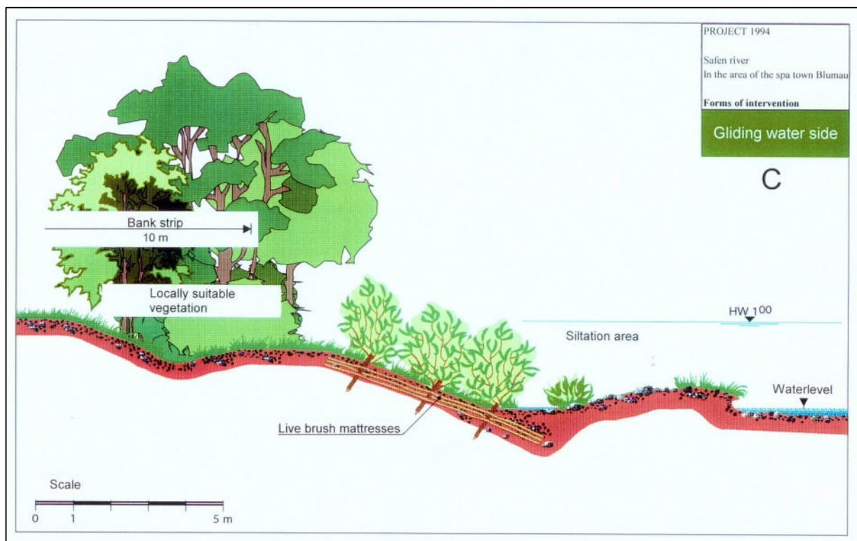
Figure 3.3.3.2.2 c - Gliding water side (type “C” measure)
