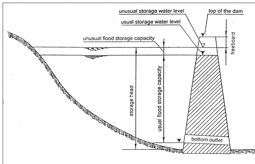
**Figure 3.3.2.2 a - Scheme of a Retention Basin**
