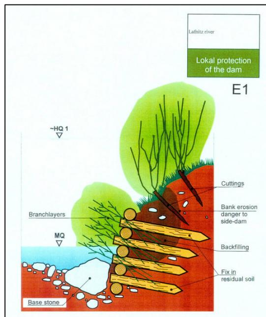
**Figure 3.3.3.2.2 e1 – Local protection of the dam (type “E” measure)**
