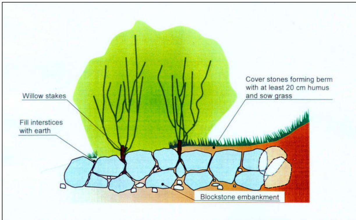
**Figure 3.3.3.2.2 f 1-** Cross section of stone groyne with cutting (type “F” measure)
