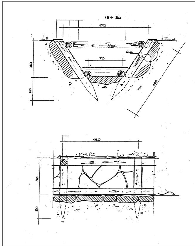
**Figure 3.3.5.3.2.2** – Scheme of a ditches made out of timber and stones
