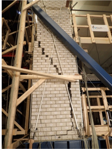
Figure 11.27: Main damage in the wide piers at the ground floor for the experiment
