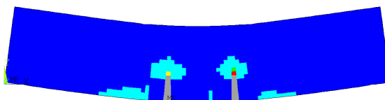
Figure 8.11: Maximum principal strain contour of the final crack pattern by SLA for the 10 MPa prestress test
