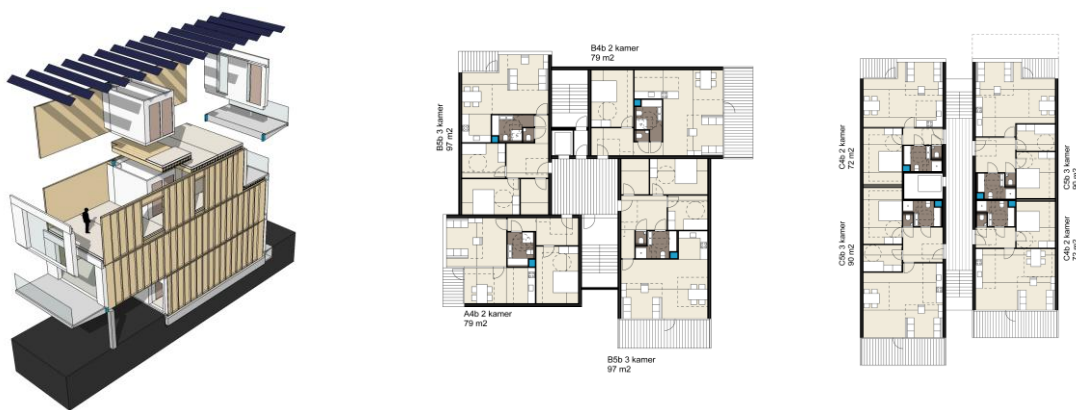
1.1 3D explosion view of a unit and different arrangements of the house units Concept House brochure
