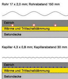
3.2.8,9 the heat distribution of the pipes and capillary mat. The Tmin (minimum temperature) is about the same as the Tm (mean temperature of the surface) at the capillary mat, although in the pipe system the difference in temperature is different. ( bioclima.de ) ( radiantcooling.org )
