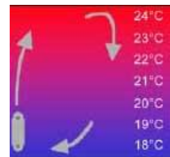
3.2.6,7 The radiation of heat or cold from the thermo active building systems from the wall or floor is even and pleasant to the human body. The heating of space with a radiator on the other hand creates temperature differences in the room ( wall-heating.com ) ( bioclima.de ) ( wall-heating.com )
