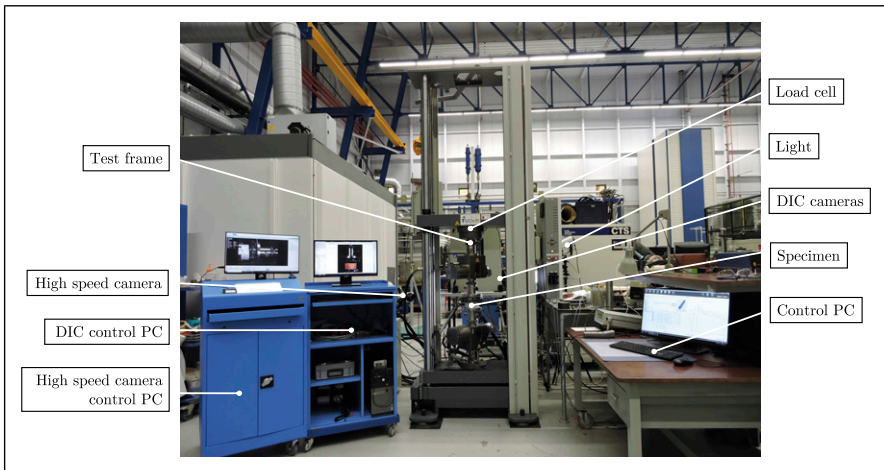
Figure 7. Test set-up at the aerospace structures and materials laboratory at the Delft University of Technology.
