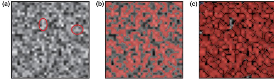
Fig. 6. (a) Two grains indicated on a Perlin texture with  $\ell = 312$  nm. (b) The grains (in red) as obtained with the *threshold* method (c) and with the *watershed* method [35]. The side length of the textures is  $10\ \mu\text{m}$ .
