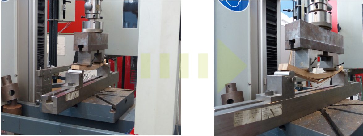
Figure:192. Bending test during test and after breaking point, always breaks at the bottom side
