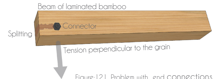
Figure: 121. Problem with end connections
