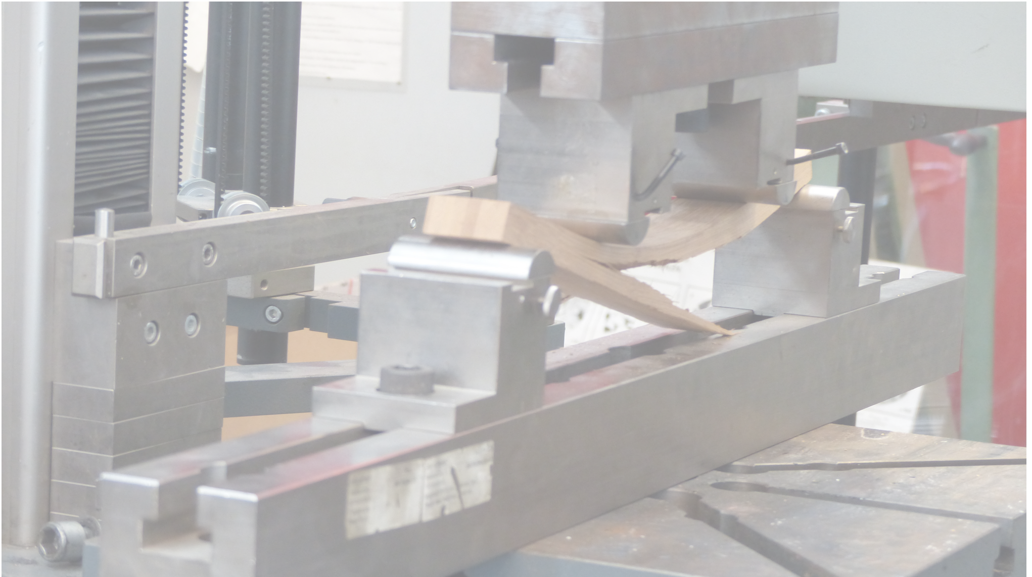
Figure: 170. Four point bending test in TU delft
