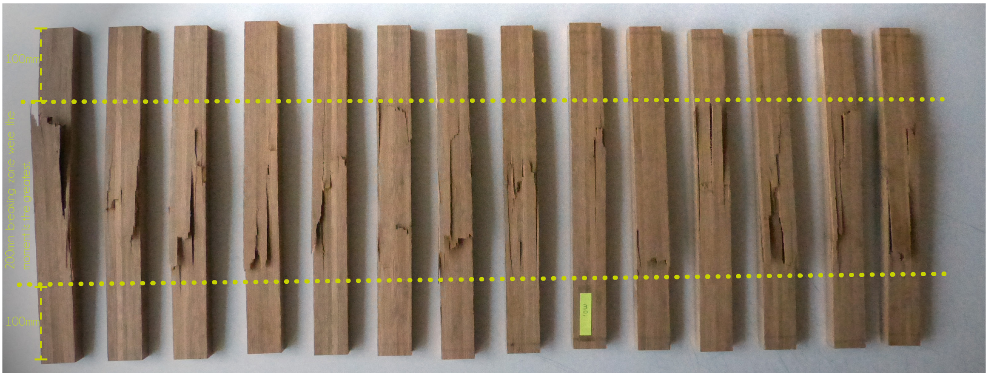
Figure:193. Sample always brakes in range a between the load point were the moment is constant and the largest, but without shear , showing that failure was caused by pure bending
