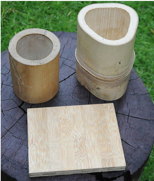
Figure:64. Triangular Guadua compared to round creates larger strips to be laminated
