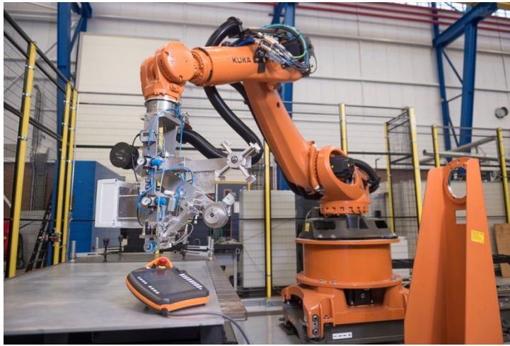
Figure 1. Overview of the KUKA automation cell with AFP end-effector
