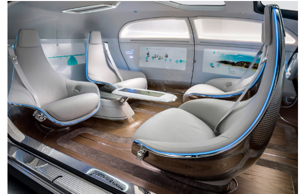
Figure 87. Interior of the Mercedes-Benz F015 concept, showing rotatable front seats.
