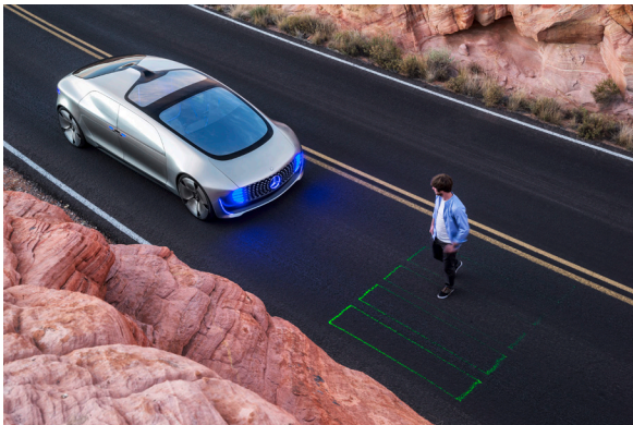
Figure 85. Outside HMI that communicates with other road users. On the left the Mercedes-Benz F015 concept and on the right the BMW Vision concept.
