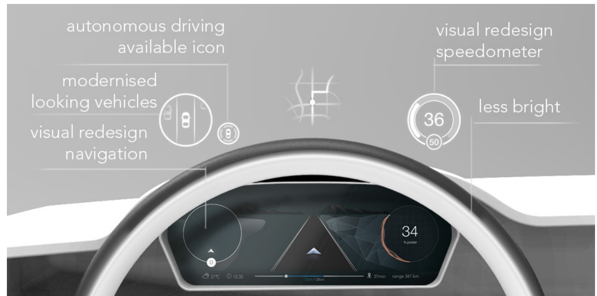
Figure 81. Redesign of the head-up display in assisted driving and navigation in the instrument cluster
