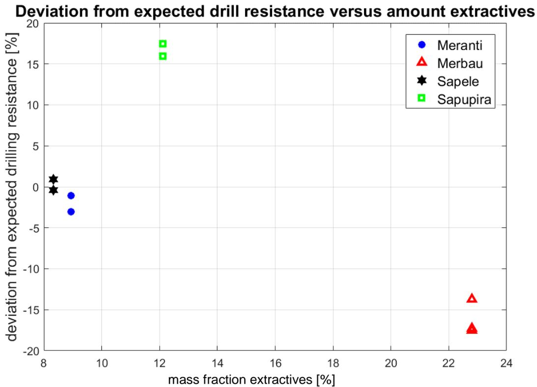
Figure 56 influence of the mass fraction extractives (% of dry mass) on the drill resistance for different tropical wood species.
