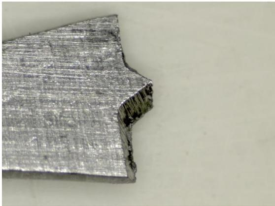
Figure 22 Microscopic picture of Resistograph drill bit (top view).
