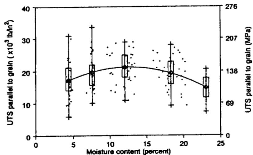
Figure 30 Ultimate tensile strength parallel to the grain versus moisture content (Kretschmann & Green, 1996).
