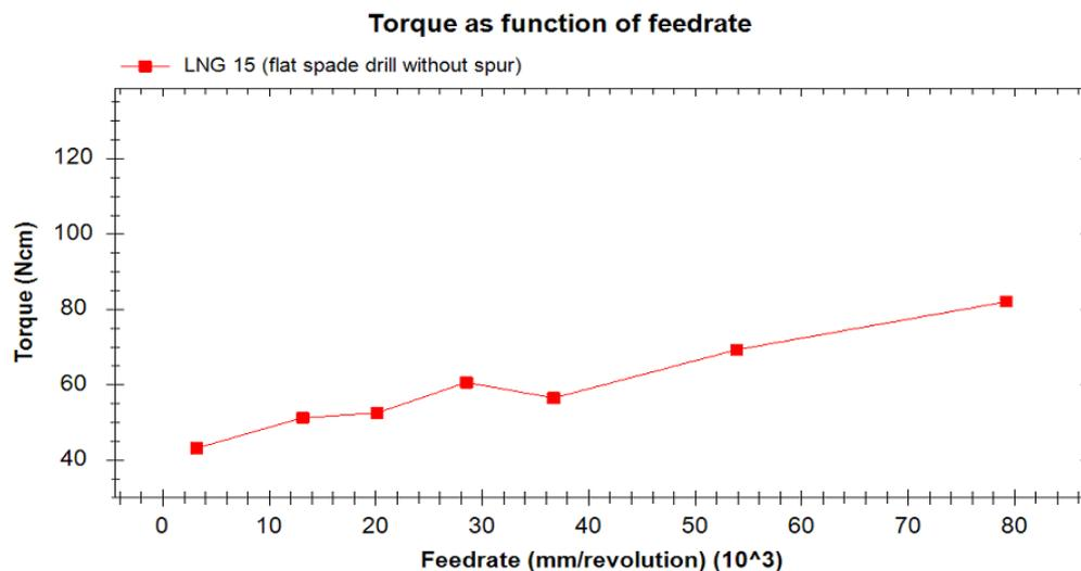
Figure 28 Torque as function of feed rate (Zhao & Ehmann, 2002) ( adapted in order to increase the visibility).
