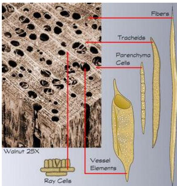
Figure 3 components of hardwood (Engler, 2009).
