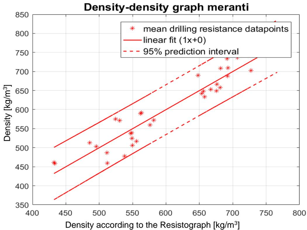
Figure 51 Calculated density versus the density obtained by measuring the dimensions and mass.
