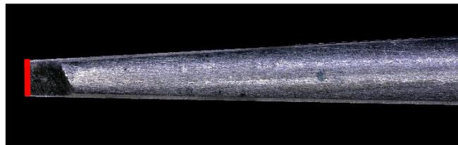
Figure 23 Side view of Resistograph needle drill.
