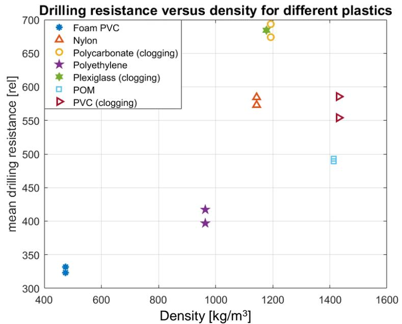
Figure 49 Mean drill resistance for different plastics
