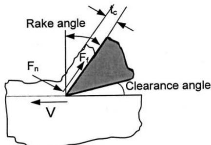
Figure 26 Chip removal model (Zhao & Ehman, 2003).
