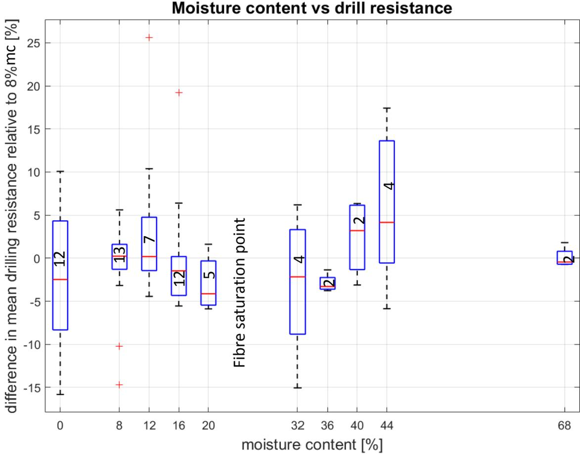
Figure 57 Influence of moisture content on drill resistance, the numbers in the boxes indicate the number of measurements between the higher and lower quartile..
