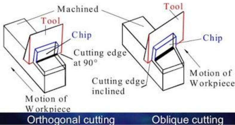
Figure 15 Difference between orthogonal and oblique cutting (orthogonal cutting and oblique cutting, 2016).
