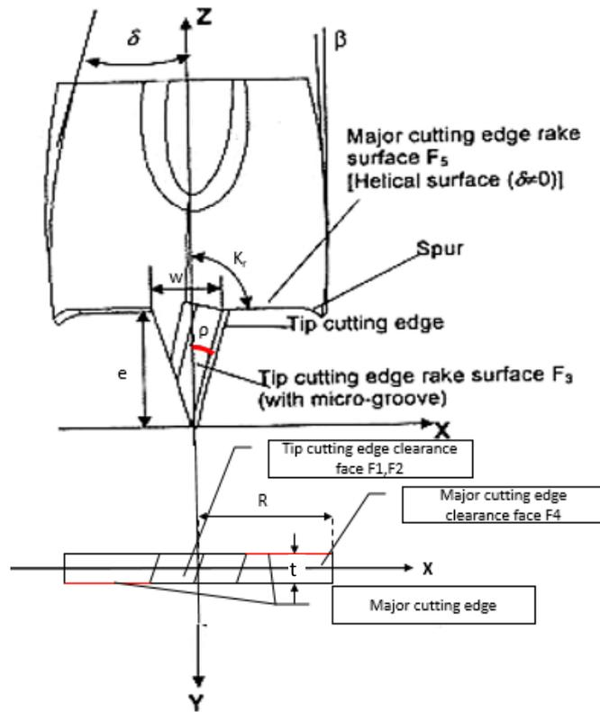
Figure 25 geometry of spade drill, adapted from (Zhao & Ehman, 2003).
