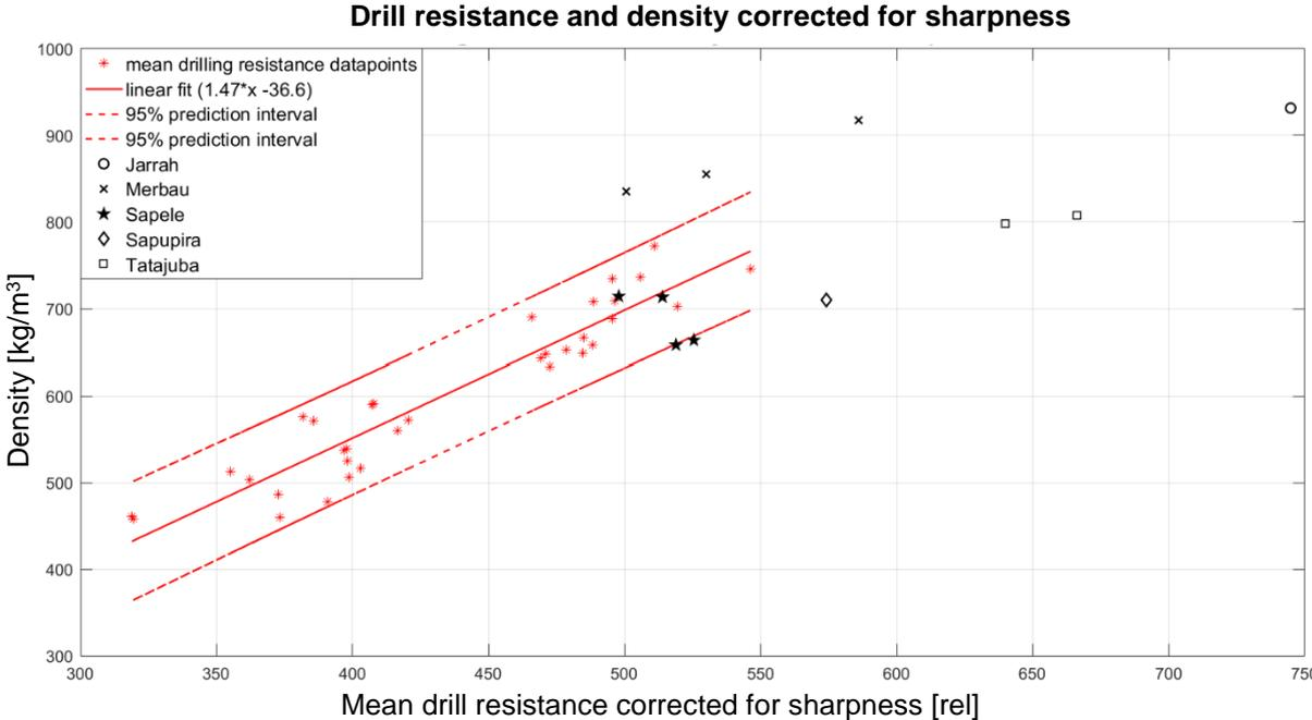
Figure 53 Drill resistance of other wood species compared to meranti, each mark in the graph represents the mean drill resistance of multiple drillings (usual three) in one sample.
