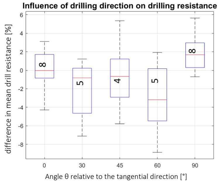
Figure 59 Influence of drill direction relative to the tangential direction on the drill resistance. The numbers in the figure indicate the number of measurements in a box
