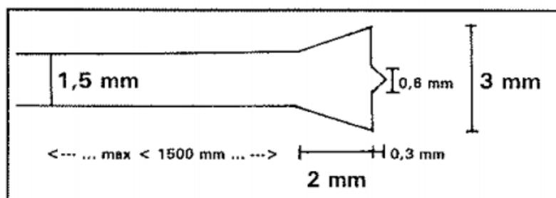
Figure 21 Dimensions of Resistograph needle drill (Rinn F. , 1994).
