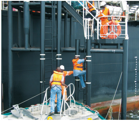
Figure 2.16: Step-over approach with the boat Landing (Bourbon Offshore, 2015)
