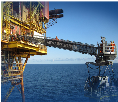
Figure 2.18: Motion Compensated Gangway transfer (Ampelmann, n.d.)
