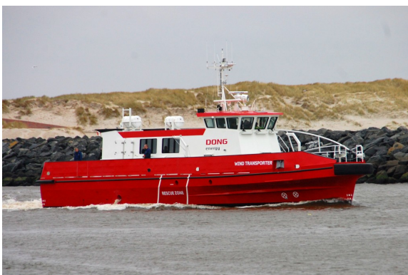
Figure 2.7: The Wind Transporter as example of a Monohull CTV (HVIDE SANDE, n.d.)
