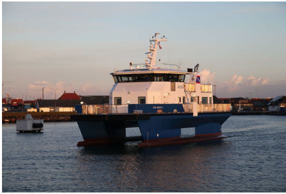
Figure 2.9: The Sea Storm as example of a SWATH CTV (ODFJELL WIND AS, n.d.)
