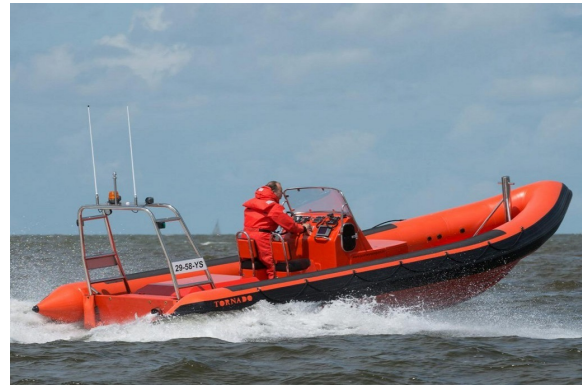
Figure 2.10: An example of a RIB as Quick Response Vessel (World Maritime News, 2012)
