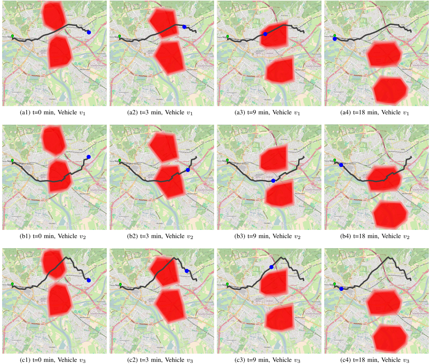
Fig. 15: Snapshots of routes calculated for 3 vehicles (in blue circle) with different categorization of risk levels. The vehicles are at the source points. The shapes and positions of the obstacles (in polygons) are the same in the three simulations, and will change as the vehicles are moving towards the destinations. (a) Vehicle v_1 , full-safe levels ={L0, L1, L2}, partial-safe levels ={L3, L4, L5}, non-safe levels = \emptyset . (b) Vehicle v_2 , full-safe levels ={L0, L1}, partial-safe levels ={L2, L3}, non-safe levels = {L4, L5}. (c) Vehicle v_3 , full-safe levels ={L0}, partial-safe levels ={L1}, non-safe levels = {L2, L3, L4, L5}.
