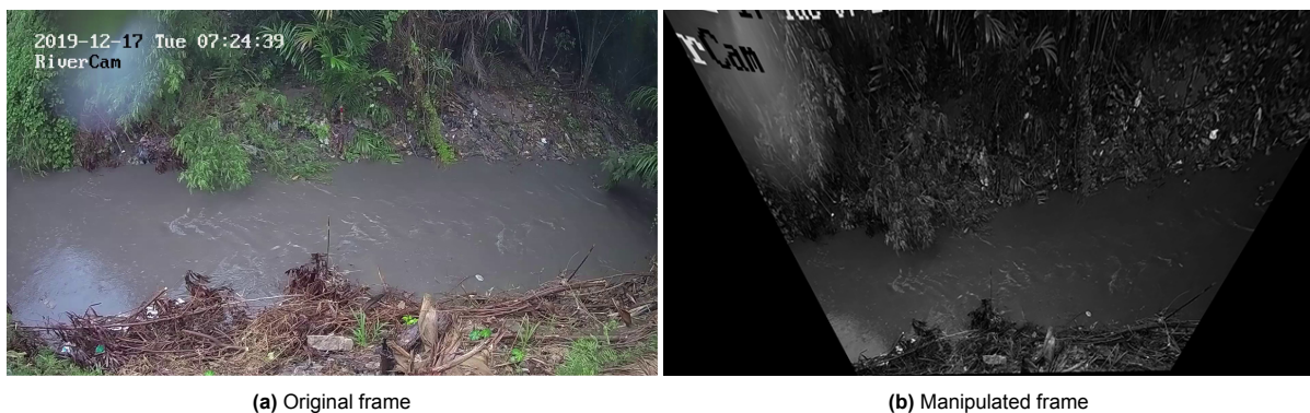
Figure 5.6: Example of the full image manipulation process for imagery obtained at the Chuo Kikuu. Sequentially, the image is lens distortion corrected, orthorectified, and turned into gray scales with additional gamma correction.
