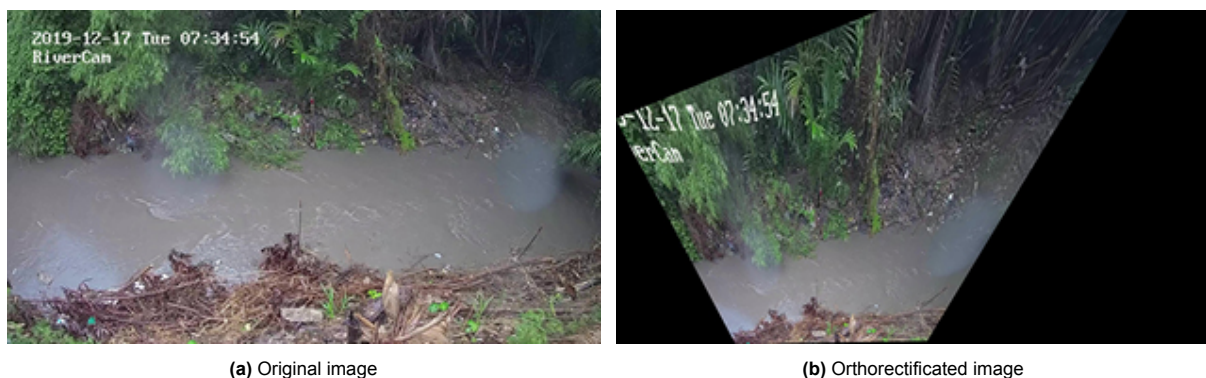
Figure 2.7: Example of the orthorectification process using four GCPs, indicated with bamboo poles alongside the stream.
