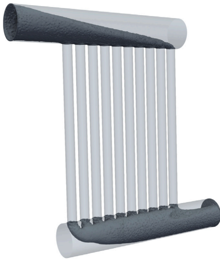
Fig. 9. Optimum geometry obtained for the cylindrical z-type manifold case using the FUA strategy, highlighting the inlet and outlet manifolds.
