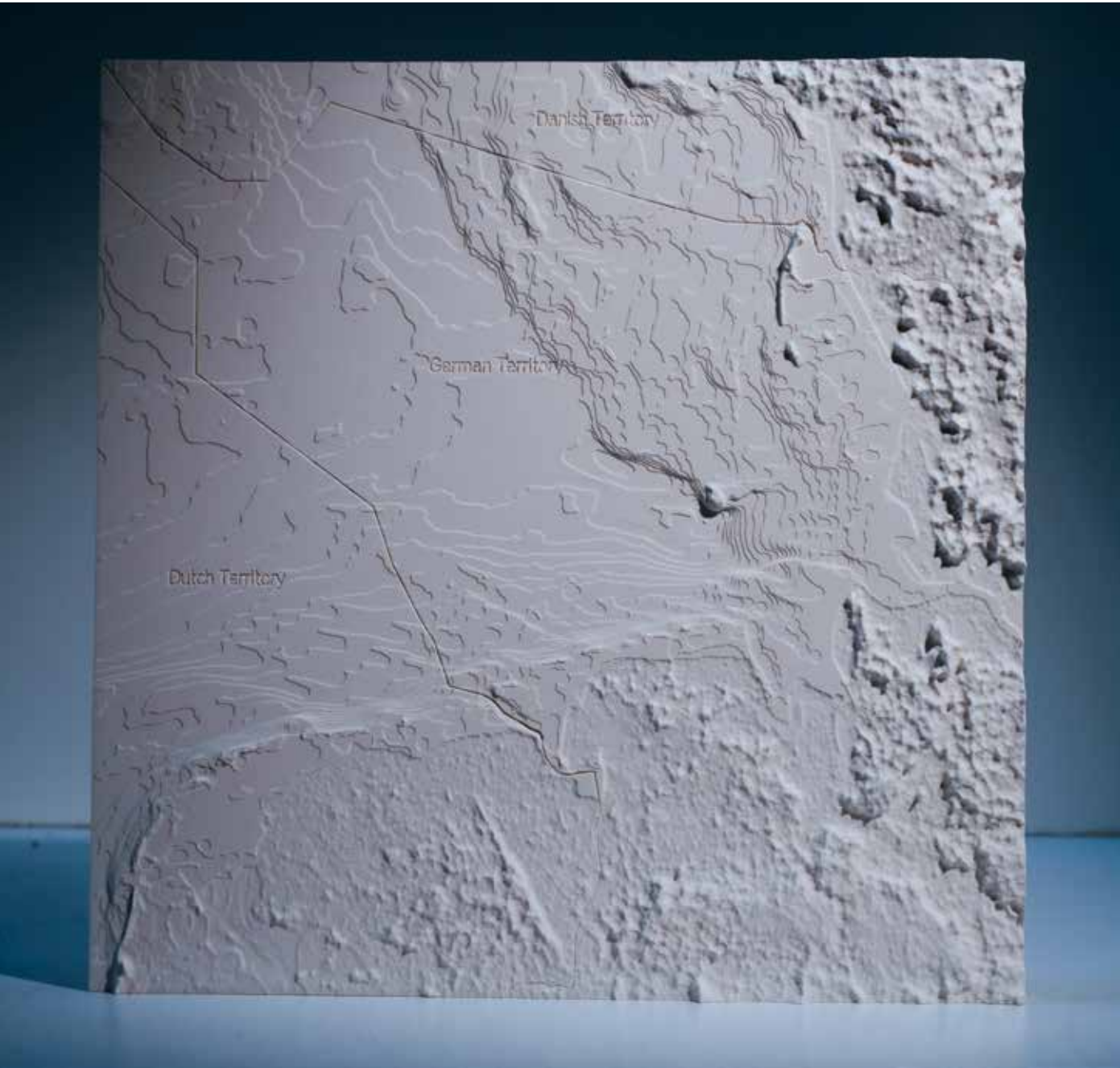
The Altitudes of Flatness, Thinking with Sections and Models Course, Year 2020-21. Horizontal scale (x) 1:750.000. Vertical scale (y) 1:7500. Model size 500 x 500 mm.
