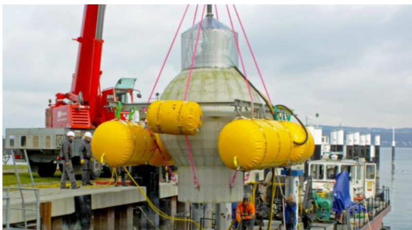
Figure A - 5 Scaled prototype of the concrete sphere used for energy storage, developed by researchers of the Fraunhofer Institute (Geuss, 2017). The yellow balloons are needed to give enough buoyancy.
