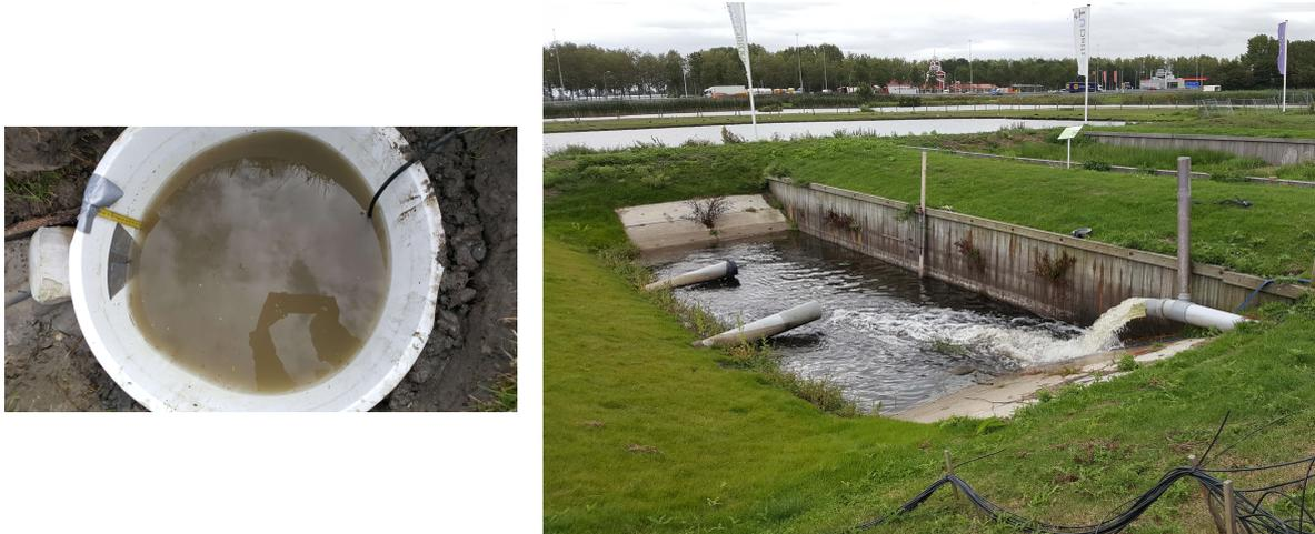
**Figure 5-3:** Left: ring (bucket without bottom) around the exit hole with a v-weir and measure tape. Right: upstream basin being filled at the start of the experiment. Entry pipes are slanted upward because of settlement of the dike.
