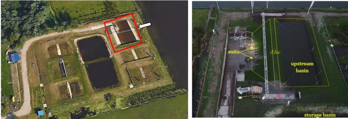
**Figure 5-1:** Left: an areal photo of the Flood Proof Holland test facility. The red square indicates the basin in which the test dike was constructed. Right: areal photo of the test dike. The upstream basin can be filled from the storage basin. The yellow lines indicate the geometry of the dike and upstream basin. Source: Pol et al. (2019)
