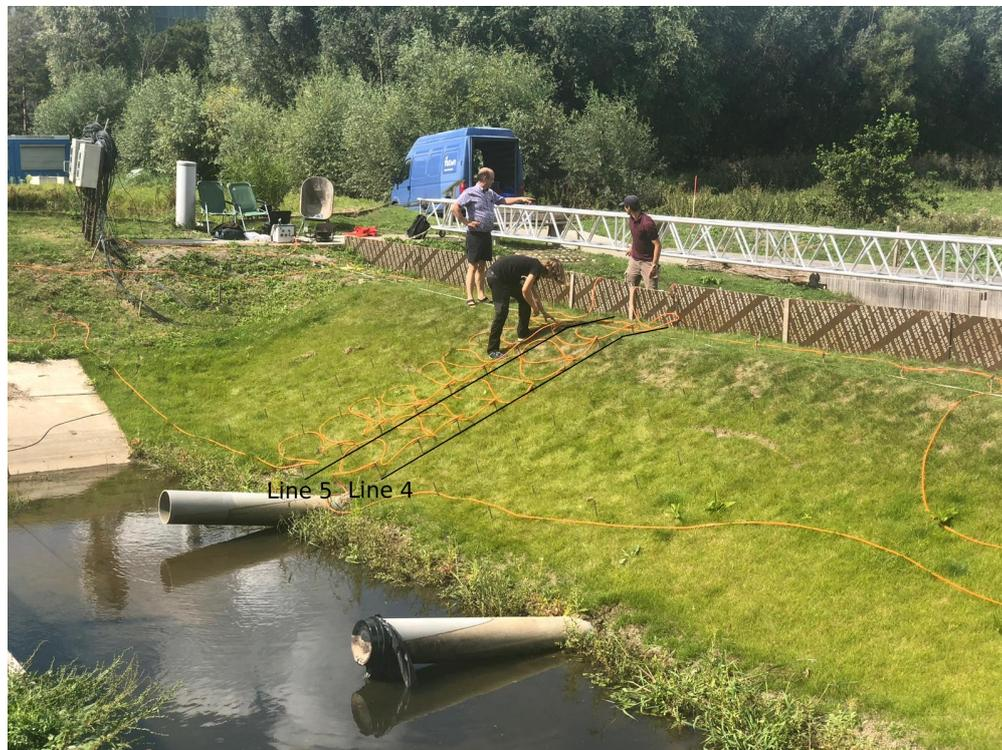
**Figure A-5:** Photo of upstream side of the dike. ERT measurements of lines 4 and 5 prior to the piping experiment.
