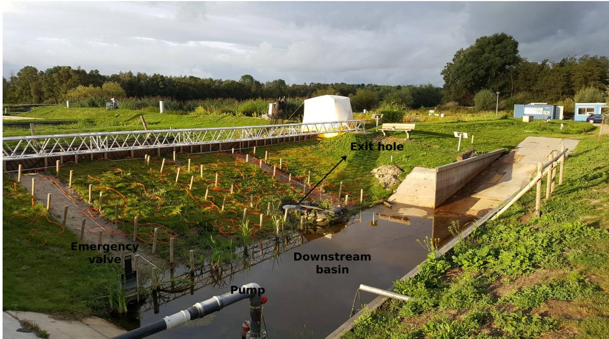
**Figure 5-4:** Photo of SP monitoring setup on the downstream side of the dike, during the piping experiment. The orange cables connected the 144 field electrodes to the IRIS instruments Syscal Pro inside the tent. Wooden poles were in place for overtopping experiments and had nothing to do with the SP monitoring system.
