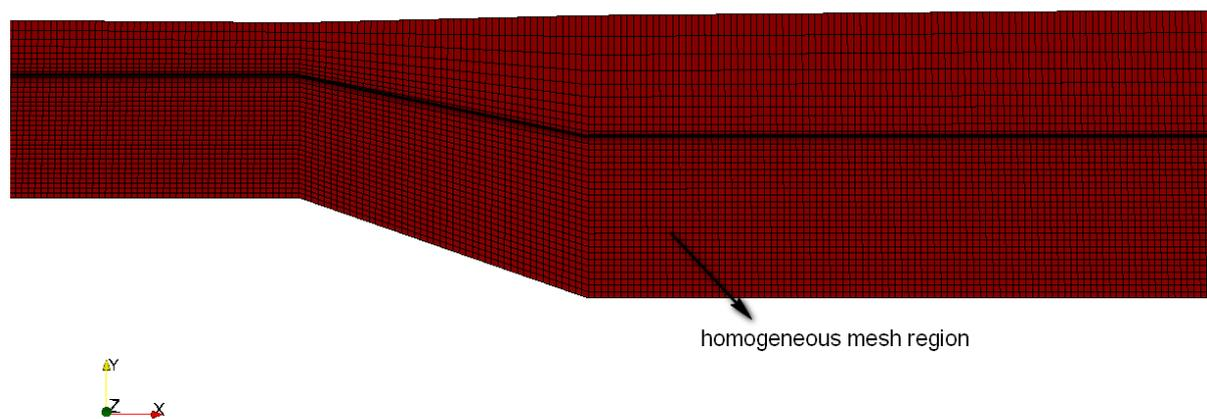
Figure 3.3: Mesh in the downstream region with indication of the homogeneous mesh region
