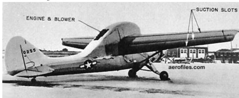
(c) Modified Stinson-Vultee L-1 'Humpback'. The hump on the fuselage houses the engine that drives the suction. [40]
