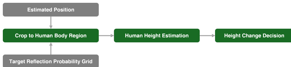
Figure 4.3: Pipeline of the proposed stand-sit classification procedure.
